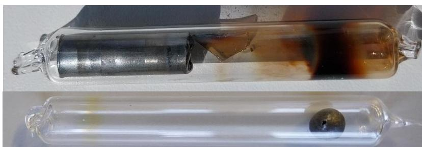
**Figure 2.3:** Filled fused silica ampoules, (top) with Ta ampoules and (bottom) with melting bead.
