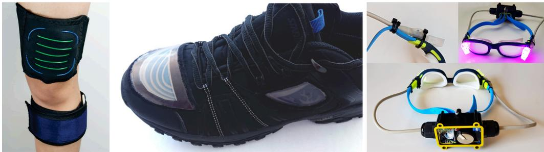
Figure 3.10: Three examples of wearable systems that use visualizations as primary output modality. Left: Electroluminescent wires integrated in a knee brace indicate the knee bending angle [6]. Middle electrochromic displays attached to the outer fabric of a shoe is used to display goals and status of the shoe [160]. Right: Swimming goggles with RGB lights in the peripheral vision of the swimmer are used as navigational aid [121].
