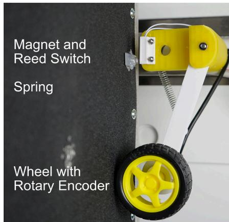
Figure 8.10: We designed a spring-loaded arm that presses a wheel onto the belt of the climbing wall. A rotary encoder mounted to the wheel measures the rotation while a reed switch detects the start of a new revolution of the belt by means of a single magnet glued to the belt.
