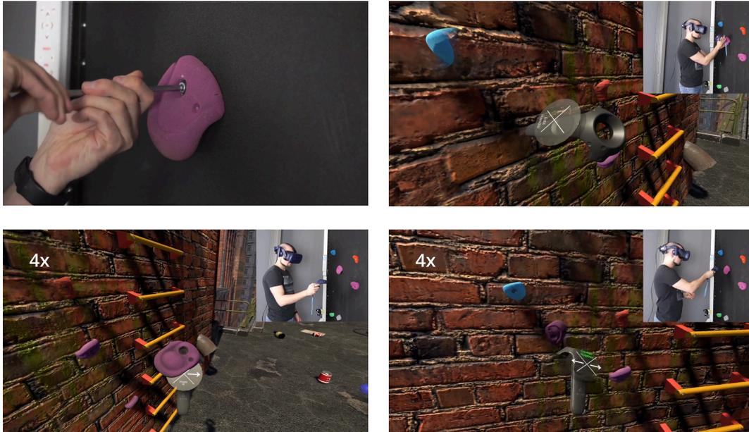
Figure 8.12: We implemented a custom editor to match the virtual holds to their physical counterparts. Based on the physically mounted hold (top left), after registering the position (top right), the virtual model needs to be selected (bottom left), to finally adjust the rotation of the virtual (bottom right).
