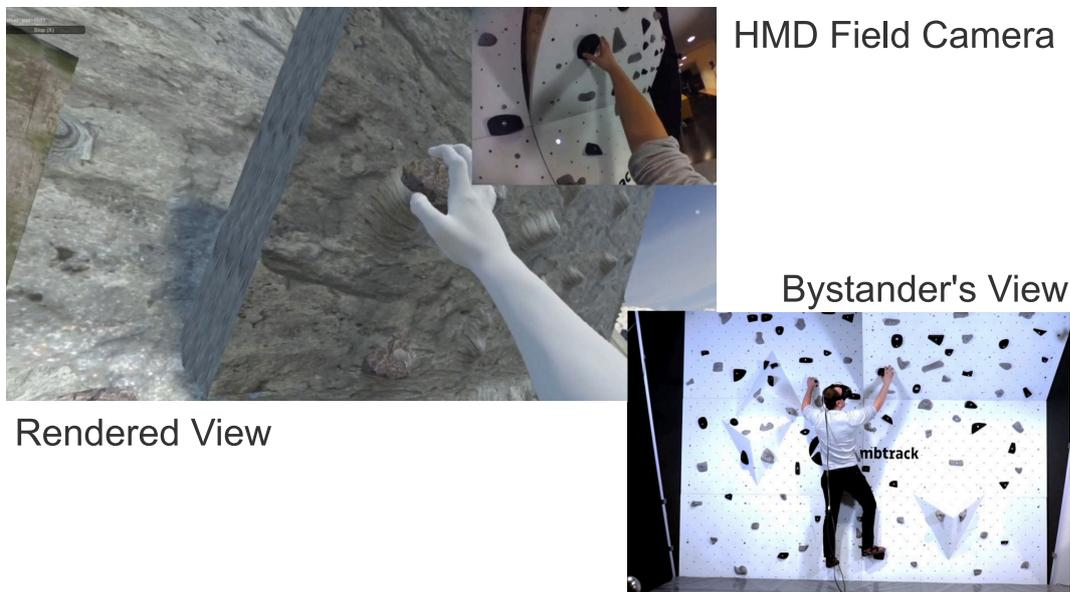
Figure 8.2: Visualization of the virtual reality climbing system. The integrated field camera of the HTC Vive was used to capture the view that the climber would have seen.
