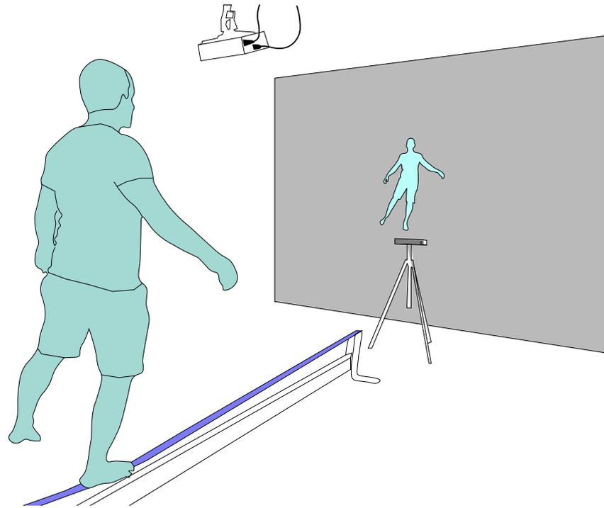
Figure 4.1: Setup of the slackline training system. The slackline is placed in front of a projected display. A Kinect facing the users tracks their movements. Real-time feedback instructs the trainee during the exercises.
