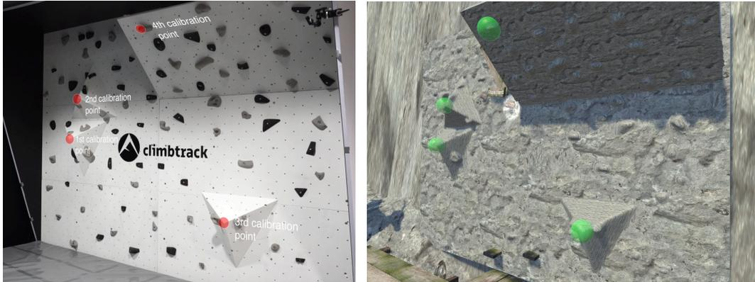
Figure 8.3: Calibration of physical and virtual climbing wall. Easily identifiable features such as climbing holds and tips of wooden volumes were used as point-pairs between physical and virtual climbing wall.
