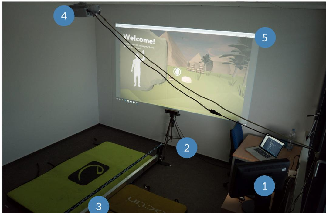
Figure 4.5: Apparatus of the user study. Slackline (3) and Kinect (2) were placed in front of a wall which served as projection screen (5). Crashpads around the slackline prevented injuries when slipping or falling. A computer (1) running the application was connected to the Kinect and a projector (4).
