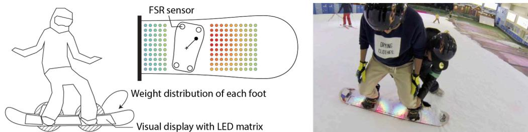
Figure 3.9: An LED matrix applied to the top side of a snowboard shows the weight distribution of the rider in real-time [177]. The visualization can be used by both, the rider and the coach.
