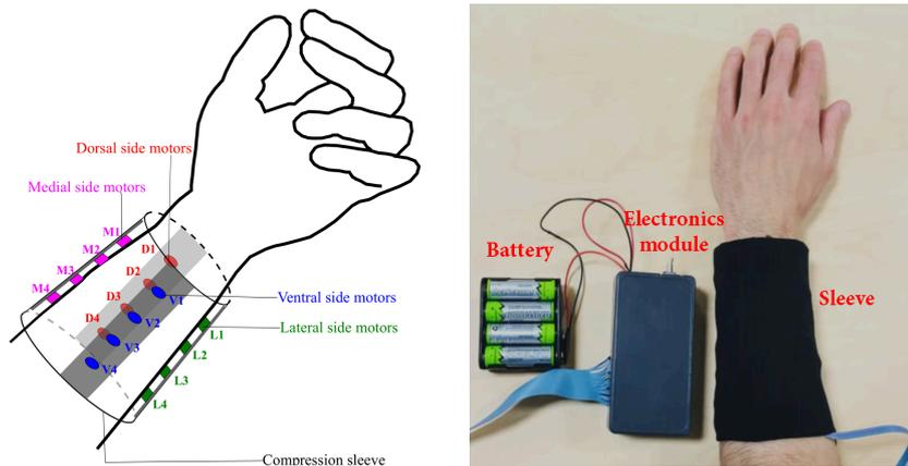
Figure 3.6: An example for a vibrotactile body-worn device capable of giving directional cues via a matrix of vibration motors placed around the underarm of the wearer [182].
