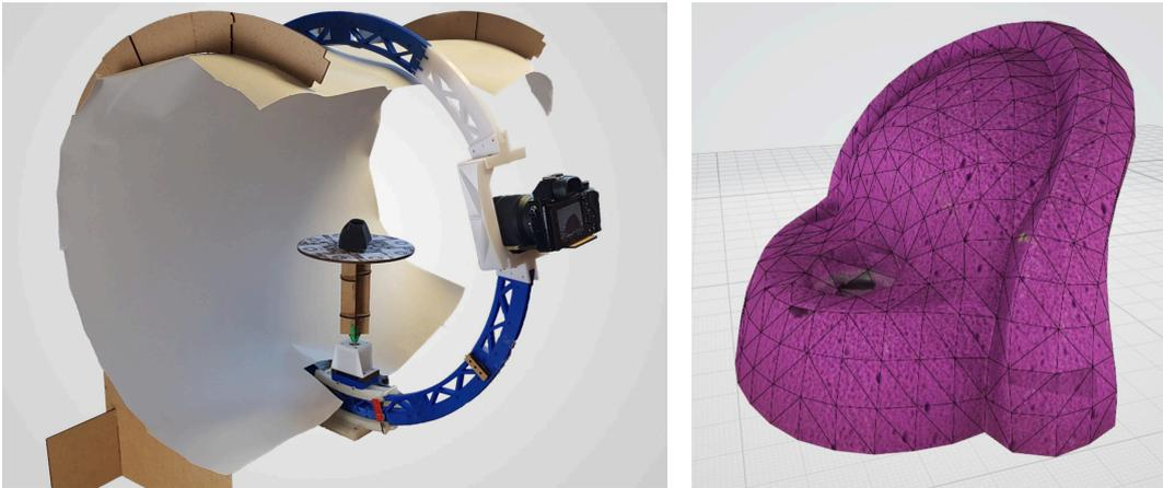
Figure 8.11: We used an open source photogrammetry rig that allows one to take a set of pictures from an object from different angles. These pictures were used in Meshroom to reconstruct 3D models of the climbing holds.
