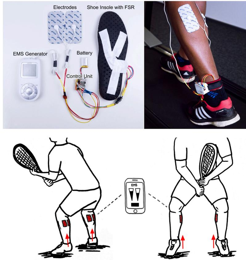
Figure 3.7: Two examples for electronic muscle stimulation of the calf muscles. Top: EMS actuation is used to actively alter the running style [97]. Bottom: Correcting the stance in racket sports [63].
