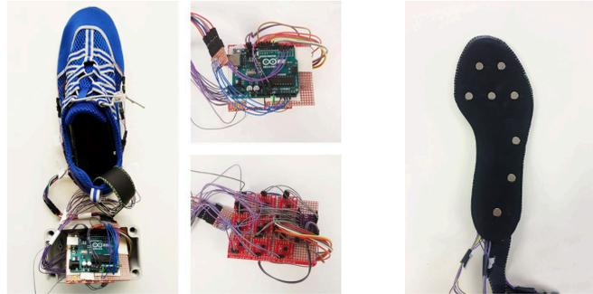
Figure 3.15: Iterative design process of a tactile, foot-worn feedback system to support weight lifting by indicating the center of pressure by means of a pressure sensitive insole. Left: Vibration motors added to the outer shell of a shoe [56]. Right: Integration of vibration motors directly in the insole [57]
