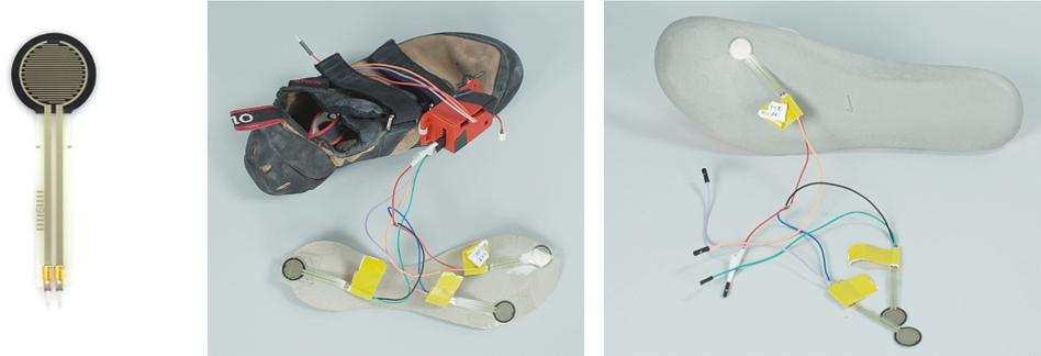
Figure 7.1: Ad-hoc smart insole applications: (Left) FSR-based sensors; (Middle) Cardboard cutout insole for a climbing shoe; (Right) Sensors applied directly to a running shoe insole.
