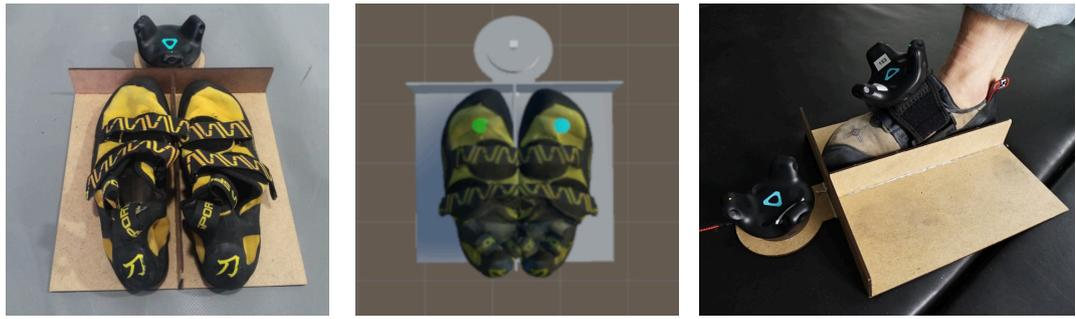
Figure 8.6: Wooden template to calibrate the climbers hands and feet with their virtual counterparts. Left: physical template, middle: virtual model of the template with 3D models of digitized climbing shoes, right: User calibration his shoe with the virtual counterpart.
