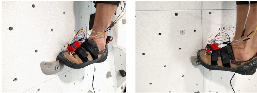
Figure 7.3: Climbing shoe with ad-hoc smart insole.
