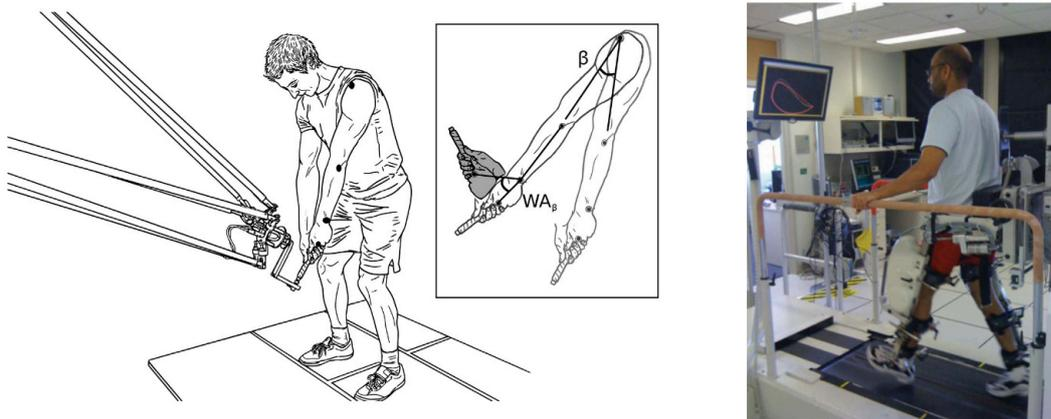
Figure 3.8: Two examples for robot aided motion guidance. Left: An endpoint controlled robot manipulating a handle of a racket [138]. Right: An exoskeleton supporting in gait training [136].
