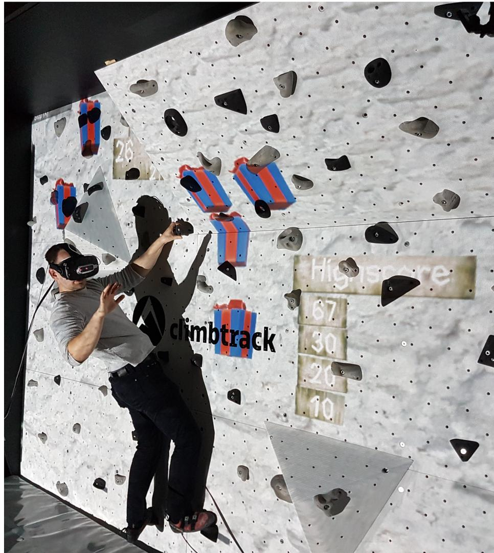
Figure 8.4: Climbing in virtual reality with a visualization of hands using the optical tracking of the Leap Motion. The virtual environment is projected back on the physical climbing wall to reflect the interactions of the player in the VE.
