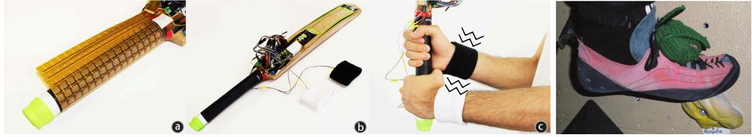
Figure 3.5: Two examples of systems providing body-worn vibrational feedback. Left: Vibration motors on the wrist provide feedback on the grip strength during a cricket pitch [162]. Right: Vibrational feedback on a climbing shoe gives insights in applied foot pressure and hasty movements [65].
