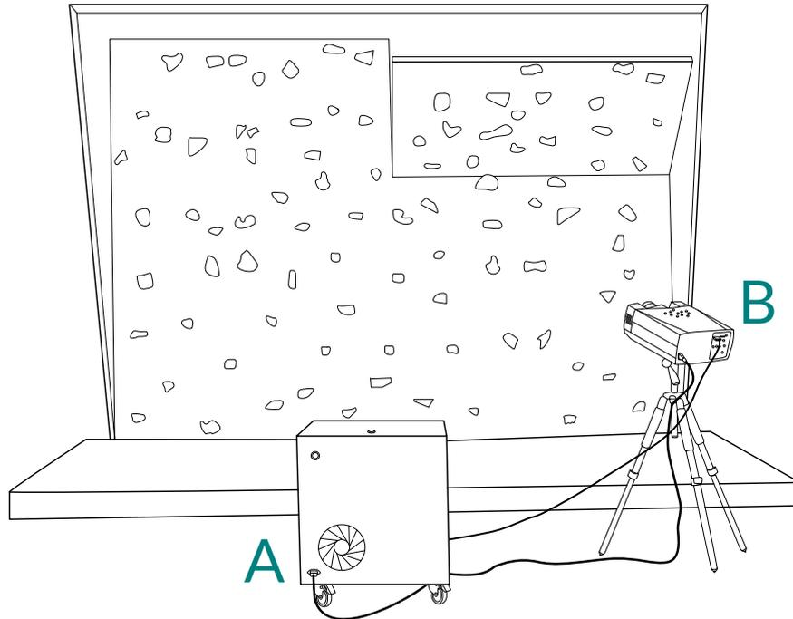
Figure 6.1: The setup of the experiment: (A) the betaCube [237] camera projection unit consisting of a projector and a Kinect V2 camera, and (B) a second projector for local, high DPI projections. Projector B could be omitted when using a 4K projector.
