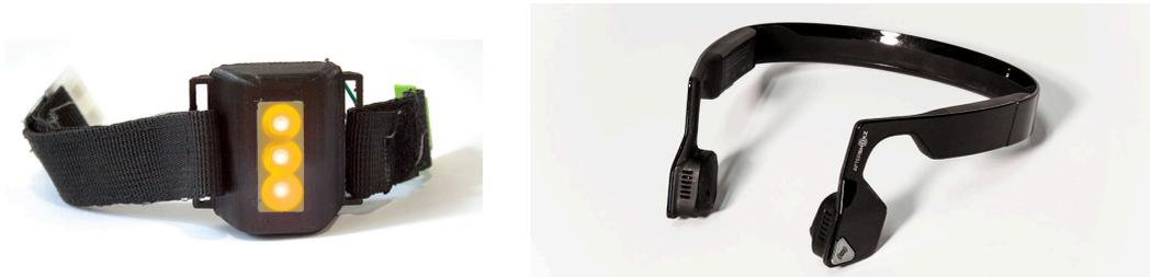
Figure 5.5: Implemented wrist-worn notification device, delivering visual and tactile notifications (left). Bone conducting headphones delivering audible notifications (right).
