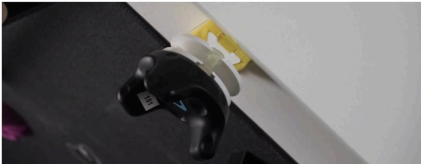
Figure 8.9: Vive tracker mounts with integrated damping
