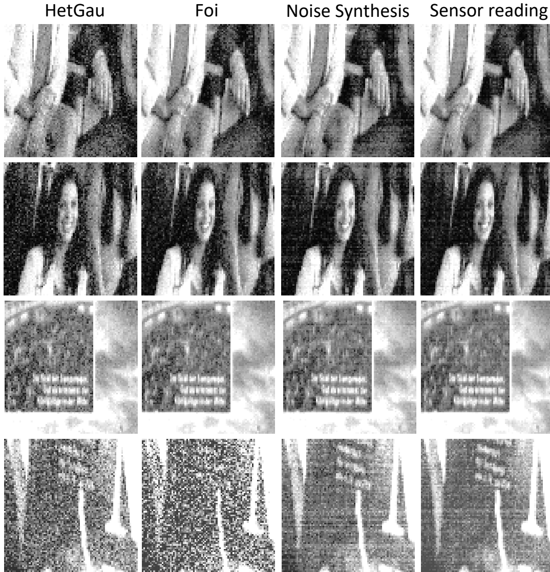
FIGURE 3.4: Given a noise-free low-exposure reference (not shown), the proposed noise synthesis is compared as well as parametric heteroscedastic Gaussian [Foi et al., 2008] (HetGau) and [Foi, 2009] noise models with a real sensor reading reference ( right column ). Note the strong correlation between the noise synthesis and the reference.
