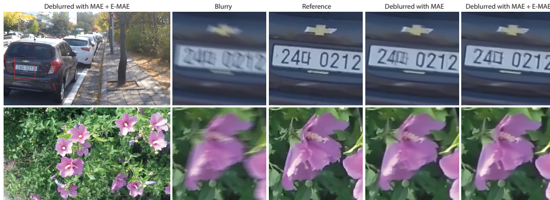
FIGURE 5.10: Visual results for the motion deblurring task when employing MAE and MAE + E-MAE as loss functions.
