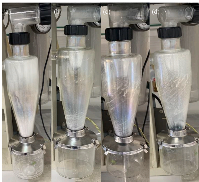
Fig. 2. Images for the cyclone with different drug-carriers with 5 % phytic acid. (a) Mannitol (b) Maltodextrin (16.5–19.5) (c) Lactose (d) Trehalose, after spray drying.
