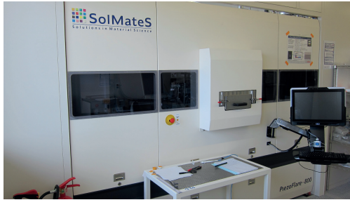
Figure 3.8. Picture of the Piezoflare 800 tool from Solmates including loadlock.
