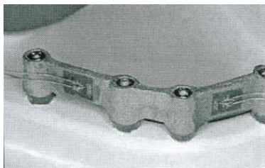
Fig. 13: Linear strain gauges are bonded on the flat surface of the connector parts of a superstructure supported by four implants. From JEMT [28].
