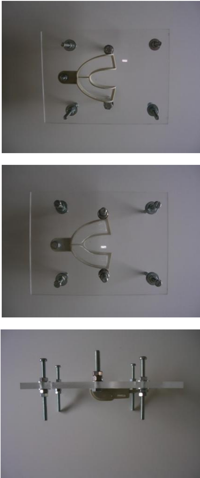
Fig. 29: Photos showing the Miratray® Implant (M) in its holding element for the impression taking procedure and for the pouring of the gypsum.
