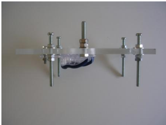
Fig. 27: Photos showing the prototype tray (K) in its holding element for the impression taking procedure and for the pouring of the gypsum.
