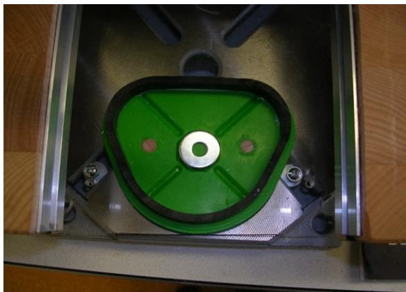
Fig. 30: The master-copy duplication system (bredent GmbH & Co.KG) and the walls of the silicone sleeve (black in the photo above).
