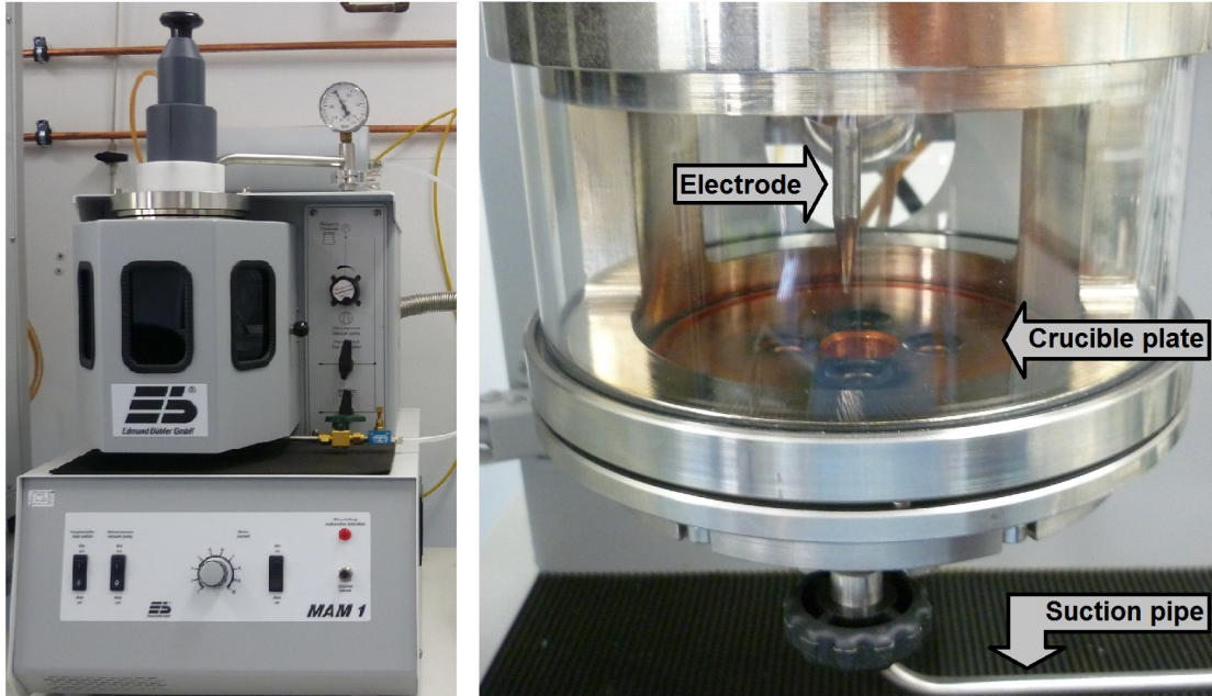
(a) left: Melting furnace of type Edmund Bühler MAM-1 with equipment for suction casting. The pump assembly, consisting of roughing pump and turbo pump, is not shown here. right: melting chamber with tungsten electrode and crucible plate. The hole in the center of the plate is where a crucible, as shown in b), is placed.
