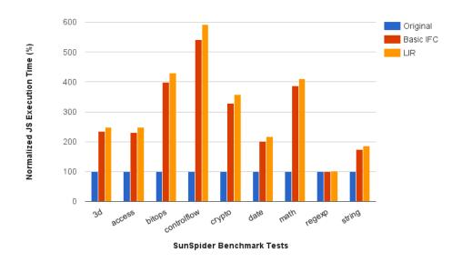
Figure 8.1: Overheads of LIR on SunSpider Benchmark Tests
