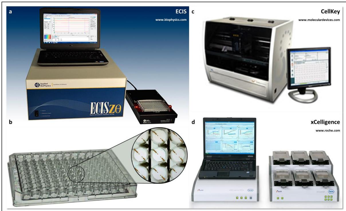
**Fig. 12: Commercially available cell impedance measurements systems:**
