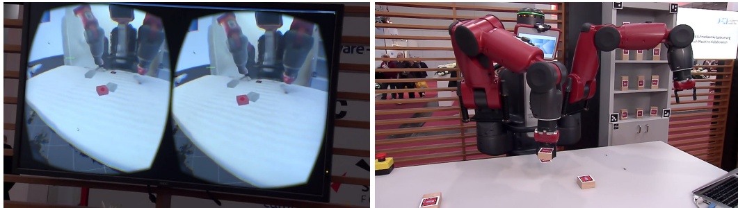
Figure 7.18: The environment setup (right) and its representation in the VR (left). The colors of the objects change when they are in the user's focus-of-attention.
