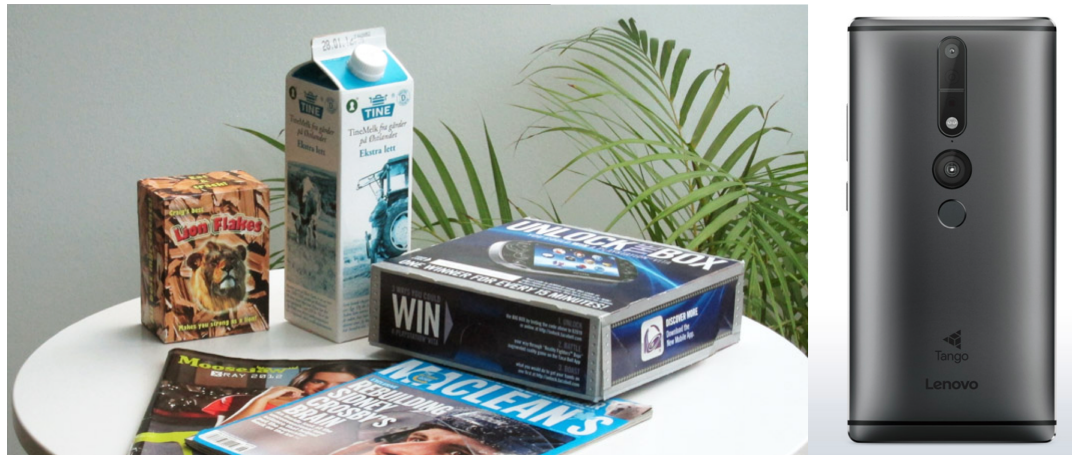
Figure 2.26: Left: Visual markers can be coded into the texture of different products. The developed application can calculate the relative 3D position and orientation toward the product. Right: A Lenovo smartphone with built in depth sensor for positioning and augmented reality applications. 29
