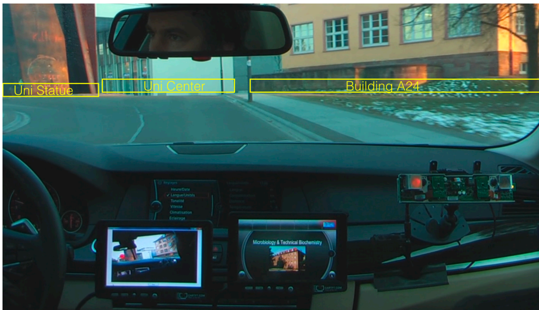
Figure 5.9: The view from inside of the vehicle. As a result of the modeling, the system sees the buildings as one stripe, regardless of their height.
