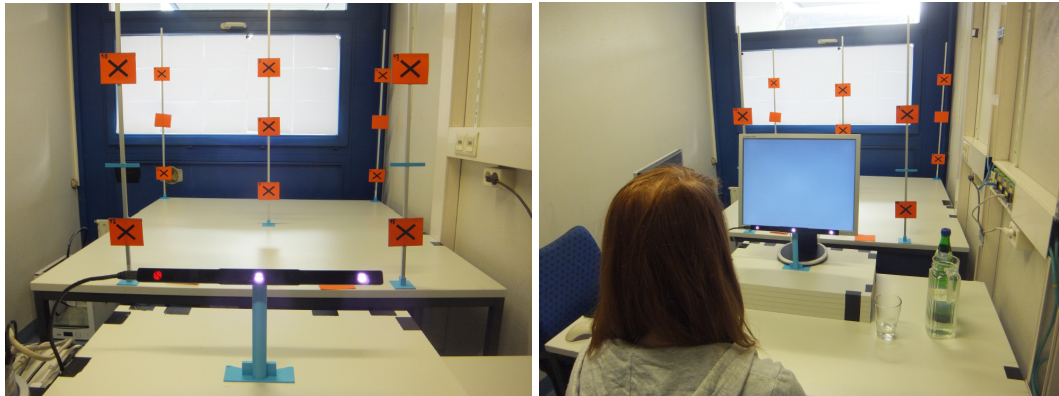
Figure 4.1: Setup for indoor eye tracking data analysis. Left: 3D analysis in room. Right: 2D analysis on display.
