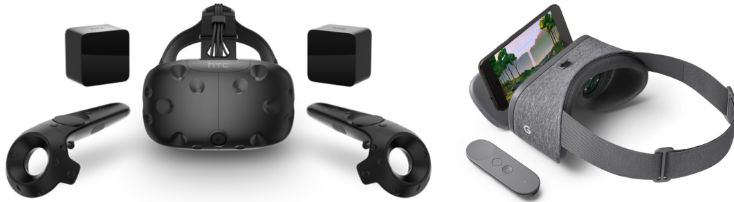
Figure 2.18: Left: HTC Vive Virtual-Reality headset. Right: Google Daydream View Virtual-Reality headset. 14
