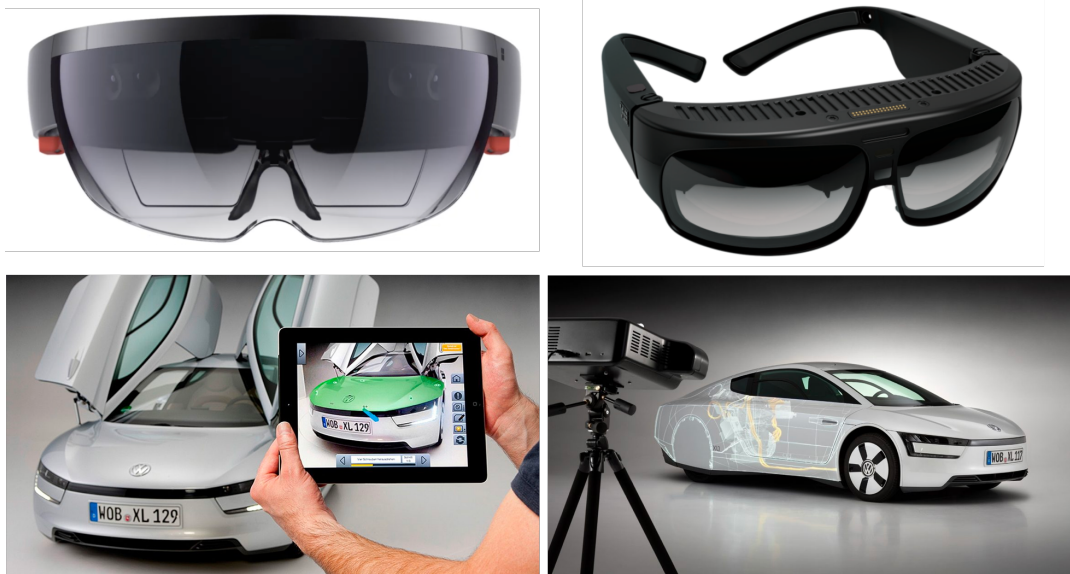
Figure 2.22: Top: Microsoft HoloLens and ODG R-9 AR glasses. Bottom: A Projection and a video see-through AR application used by Volkswagen AG for the XL1 model. 15
