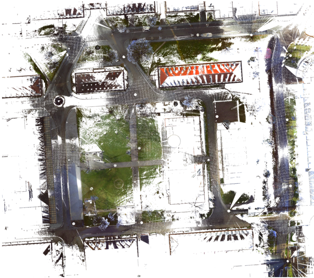
Figure 5.12: Upside view of the 3D point cloud of the Saarland University campus. The small circles represent the scanning locations.
