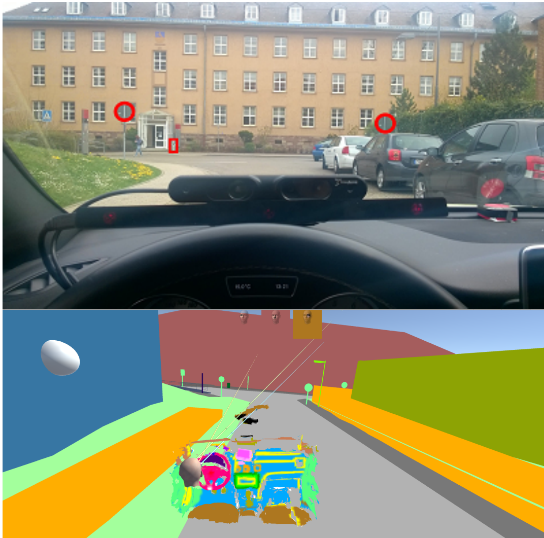
Figure 6.2: An example scene for interaction in outdoor environments containing three target objects. The environment model, the vehicle model and the direction of the focus are all integrated in one environment. The rays represent the direction of the eye gaze and head pose.
