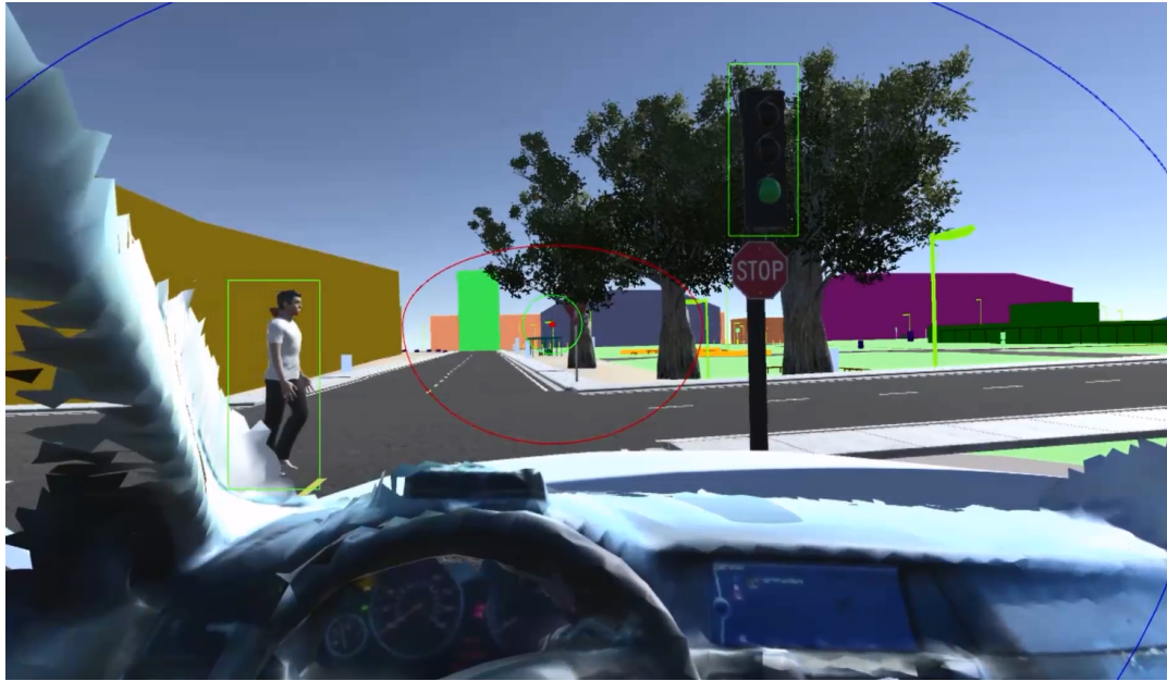
Figure 7.28: The simulated automotive use case: the visibility of relevant objects (pedestrian, traffic light) in the peripheral view of the driver serve as input for assistive system functions (attention shift).
