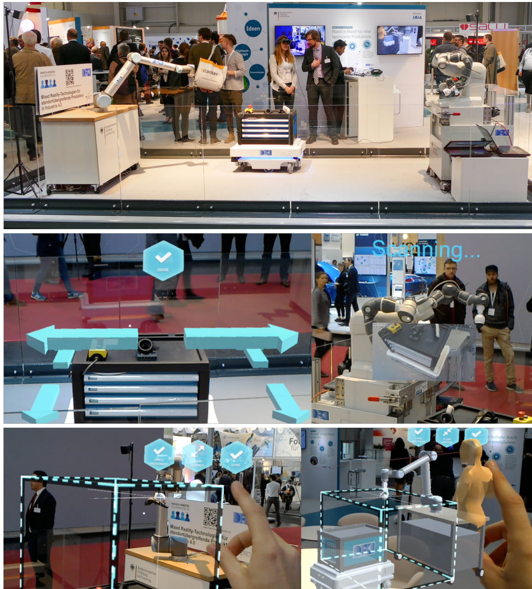
Figure 7.23: Top: An Example setup of the developed scenario for Mixed Reality Human-Robot Collaboration. Center: Interaction with MiR100 and the ABB YuMi. Bottom: Interaction with UR10 as in the vicinity of the robot (left) and from a distance (right).
