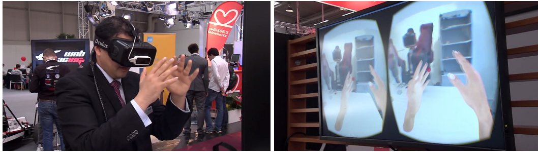
Figure 7.20: The setup for the user which monitors the environment through VR. The detailed hand movement of the user is also integrated into the environment.
