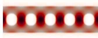
(c) Mode profile of the dielectric band at the X-point.
