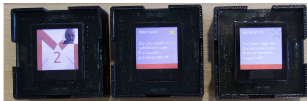
Figure 2.8: Creating an interactive surface of a variable size by placing CloudDrops close to each other
