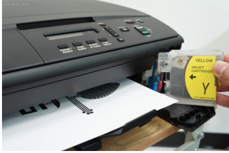
(a) Fast fabrication of printed traces using an off-the-shelf printer filled with conductive silver ink [33].
