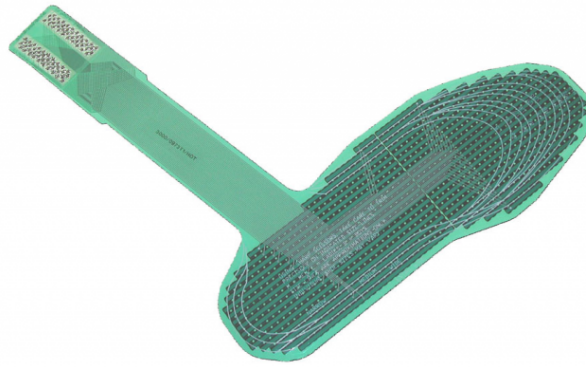
Figure 3.12: Tekscan [113] is a pressure sensor for shoe insoles. It can be cut along the predefined silver lines to fit the size of the foot.
