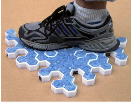
(a) Building sensate floors out of multiple pressure sensitive Z-Tiles [85].
