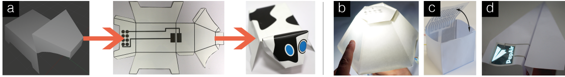
Figure 5.1: Foldios are designed in 3D. Print & fold layouts are automatically generated, including customized printable electronics for sensing and output. The technique enables quick, easy and inexpensive fabrication of a wide variety of folded interactive objects, including b) UbiComp devices, c) actuated shape-changing objects and d) lightweight paper crafts.
