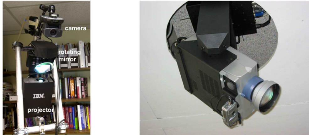
Figure 3.2: Two solutions to create Steerable Projectors - On the left side the Everywhere Displays approach by Pinhanez where a steerable mirror is positioned on top of the projector to deflect the projection ray [164]. On the right side the beaMover approach, where a projector is rested on a moving head to redirection it's output [35].
