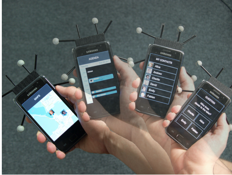
Figure 6.3: mSpaces - Spatially-aware mobile device. Different workspaces appear depending on the devices position.
