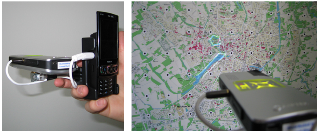
Figure 4.5: Map Torchlight - The hardware prototype used for Map Torchlight (left) and the augmentation of a paper map using Map Torchlight (right).
