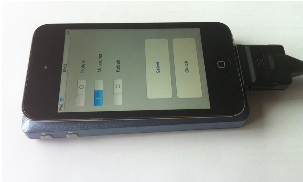
Figure 6.13: Dynamic Peephole Prototype Device - The prototype consists of an 4th generation iPod Touch and a Microvision ShowWX Laser Projector.
