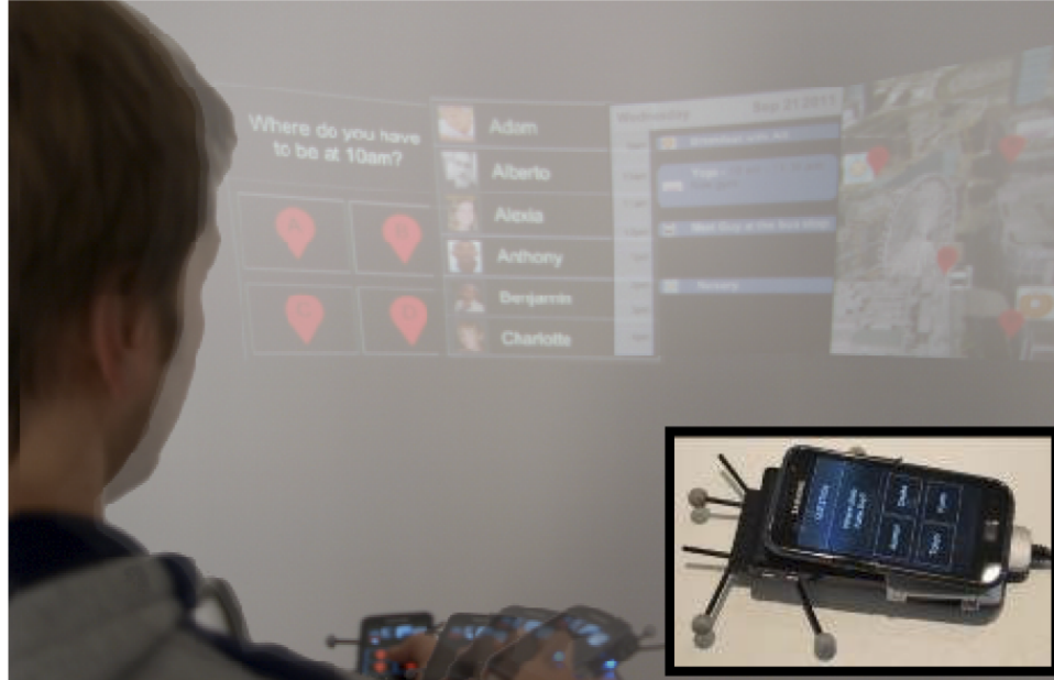
Figure 6.1: pSpaces - User accesses various virtual workspaces by moving the pico-projector to the associated physical space.
