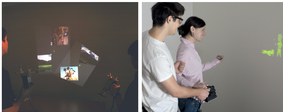
Figure 3.8: Multi-User Interaction with Hand-Held Projectors - On the left the system of Cao et al. merging multiple projections in one information space [38]. On the right the Side-by-Side system allowing multiple users to interact with multiple projectors without any instrumentation [215].
