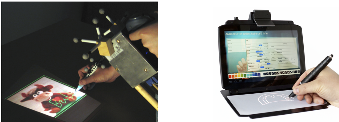
Figure 3.13: Pen Input on the Projection - Left: Cao and Balakrishnan used a Vicon tracking system to track projector and pen to allow for intuitive input [37] Right: The PenBook uses an Anoto pen for interaction on the projection [224]
