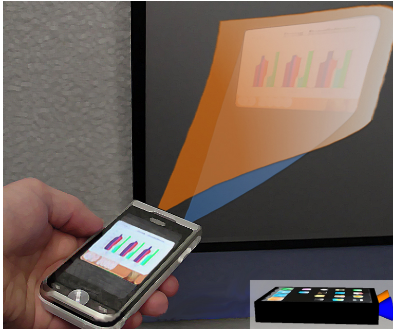
Figure 4.3: Congruent alignment of camera and projector - The FoP is completely included in the FoV
