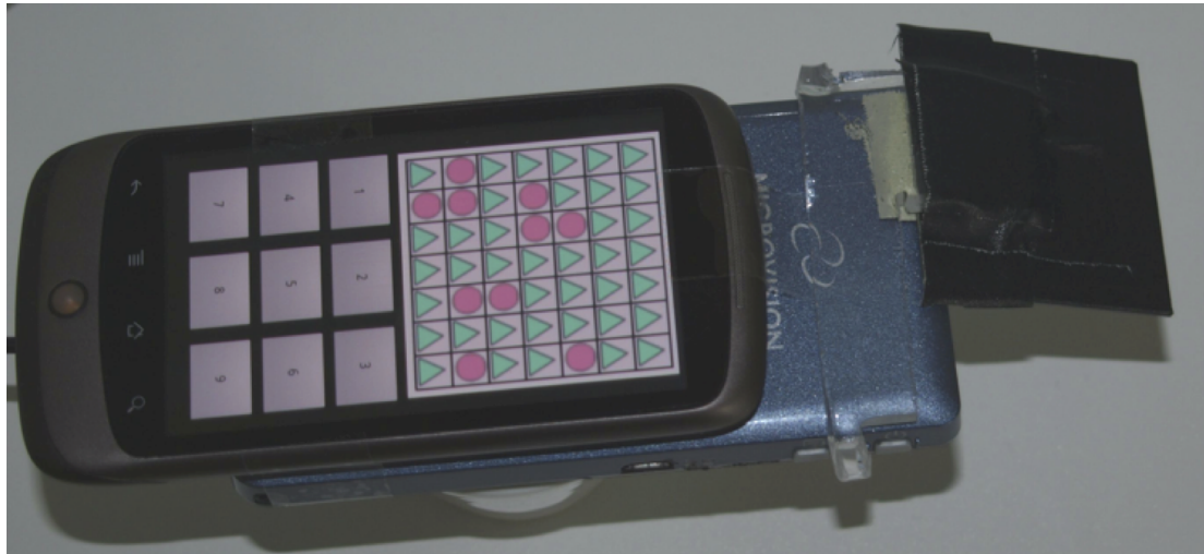
Figure 5.4: User Study Hardware - Phone and projector used for the user study fitted with the Floor setting mirror
