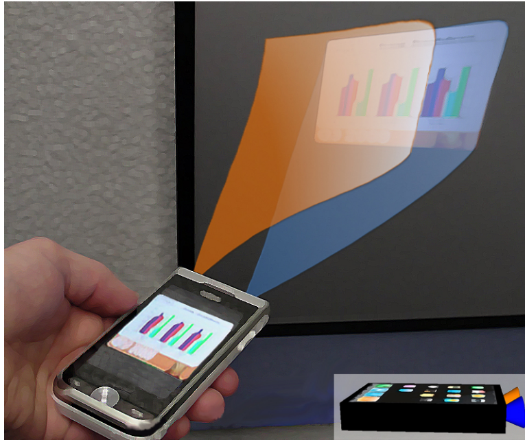
Figure 4.2: Partially intersecting alignment of camera and projector. - The FoV and FoP are partially overlapping each other.
