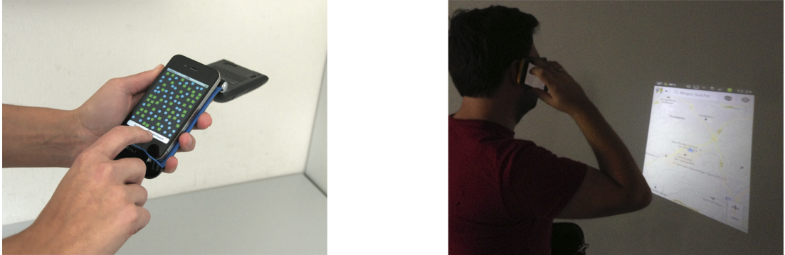
Figure 3.14: Input on the projection device - Left: Current projectorphones and detachable projection cases rely only on input on the touch-screen of the device [165]. Right: An interaction technique to allow in-call interaction directly on the projecting device [129].
