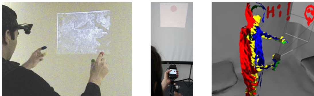
Figure 3.18: Interactions around the projecting device - Left: The SixthSense system allowed for gestures executed between the projector and the projection surface [146]. Center: Winkler et al. analysed different mid-air pointing techniques using an optical tracking system [221] Right: Such mid-air pointing techniques have been implemented by Molyneaux et al. [149]
