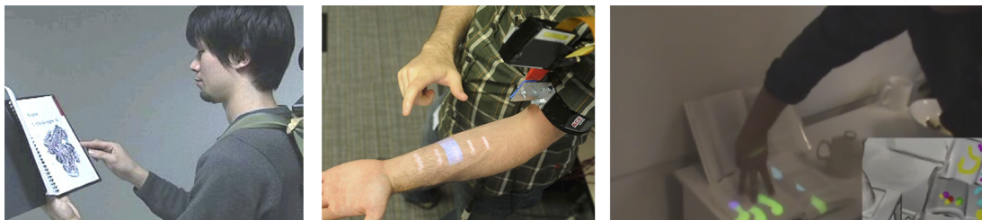
Figure 3.12: Direct Touch Interaction on the Projection - Left: Karitsuka and Sato presented a system that employed a infrared reflective finger cap to register touches [104] Center: Harrison et al. used muscle sensing techniques to detect on body touches [85]. Right: Based on an environmental model Molyneaux et al. identified the position in the projection the user is touching [149]
