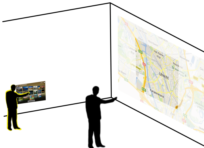
Figure 7.1: Distribution of applications around the user - A user interacting with two different applications at different positions with different interaction techniques. When being closer to the wall the user can touch the projection (yellow) and when being further away the user can use a dynamic peephole projection.
