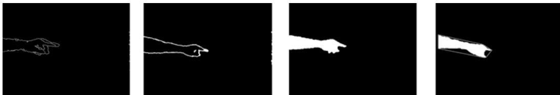
Figure 7.4: Processing pipeline for touch detection - Steps of the hand detection algorithm based on the depth image. From left to right: Canny Edge detection, Determine Contours after Dilation and Erosion, fill Contours, determine convex Hull.
