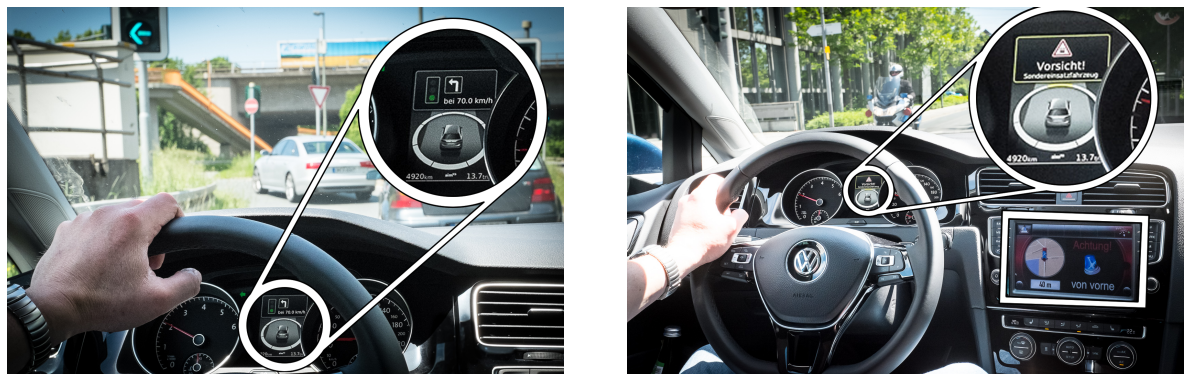
Figure 10.2.: PADE's presentation component integrated into the Volkswagen Golf VII. An additional display strategy representing the multifunctional display was added to the presentation model. Left: traffic light assistant; right: emergency vehicle warning. (Image reproduced with the permission of Volkswagen AG.)
