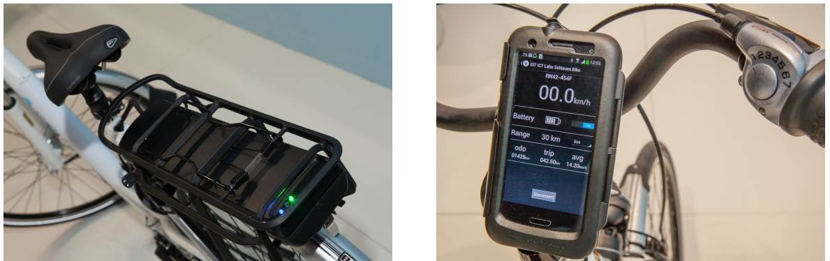
Figure 10.4.: E-bike fleet management demonstrated at the Mobile World Congress 2013, Barcelona, Spain. Left: battery with status LEDs; right: smartphone connected to the bike with controls for the bike’s battery.
