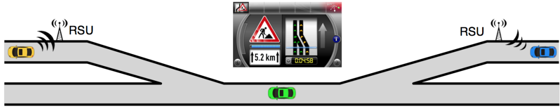
Figure 3.5.: Roadworks information system in \text{sim}^{\text{TD}} . The yellow car delivers data from vertical acceleration sensors to an RSU when leaving the work area. Its geometry is computed and transmitted to the blue car entering the roadworks. While driving through the roadworks, information on geometry, traffic flow and estimated time to end is displayed. The image in the middle shows the visualization within \text{sim}^{\text{TD}} for the green car.
