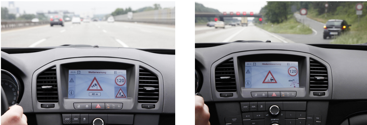
Figure 10.3.: PADE's presentation component integrated in an Opel Insignia. It consisted of a main screen and a symbol area with two slots that were arranged vertically. Left: road weather warning on the main screen and traffic sign assistant as well as roadworks information system on symbol area. Right: broken-down vehicle warning on main screen and traffic sign assistant on symbol area. (Image reproduced with the permission of Opel AG.)
