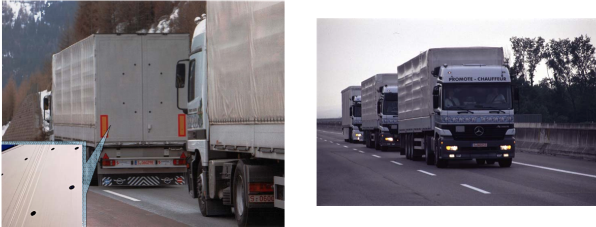
Figure 2.2.: Trucks used in Chauffeur II for the platooning application. On the left picture, the active infrared pattern used for tracking is clearly visible.
