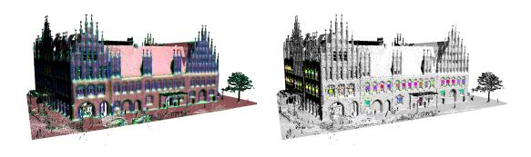
**Figure 7.21:** Structure retrieval – 1st step: We use the directed orientation histogram descriptor (left) and use 4 windows (each form a different class) to train a multi-class window model. For each found window instance we generate the descriptor for the next hierarchy level. The colored centroids represent the resulting descriptors after projection onto the first principal components. Please note windows of the same type inherit similar colors.
