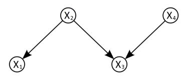
**Figure 4.2:** A simple example for a Bayesian Network with variables  $X_1, \ldots, X_4$ .  $X_2$  and  $X_4$  are independent,  $X_3$  is dependent on  $X_2$  and  $X_4$ , whereas  $X_1$  is only dependent on  $X_2$ .
