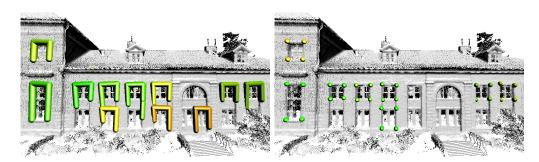
**Figure 7.13:** Comparison to the Markov chain model in Chapter 6. Because of the lacking global correlations, lower boundaries of the windows do not match up (left), which the fully-correlated model avoids (right). For both examples identical training instances are used. Edges encode the chain used in the previous approach.
