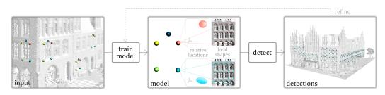
**Figure 7.2:** Outline of the method. Given sparse user annotations defining some shapes and their correlations, a shape model characterizing these shapes is constructed. Each node in the model is associated with corresponding distributions for the local shapes (descriptors) and the relative location within the shape. The efficient detection allows for refining the model interactively.
