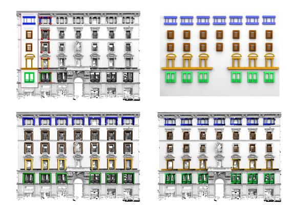
**Figure 6.19:** The detected object correspondences are used to align synthetic 3D models with detected objects of different (color coded) categories. The upper left shows the training examples and the matching primitives. The lower left shows all detected shapes. The right side shows the aligned primitives.
