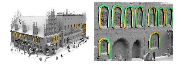
**Figure 6.14:** Single-class learning: Detecting "all windows". Training data (blue spheres) consists of only 4 exemplar windows. Left: Without scaling the learned covariance matrices the results deteriorate compared to Figure 6.13. Right: Detail of overlay: green (unscaled), yellow (scaled). When using scaled versions of the learned covariance matrices, the extracted instances adopt better to the underlying geometry. Without scaling the noise level exceeds learned correlations.
