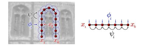
**Figure 6.3:** Objects are modeled as Markov chains: Each node is controlled by a potential function  $\phi$  that matches local shape. In addition, pairwise potentials  $\psi$  encode the variations of the spacial alignment of parts.
