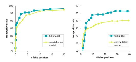
**Figure 7.10:** Comparison with constellation model: The detection rate improves by including descriptor correlations. The left diagram shows results for the specific class of rigidly similar windows, the right for the more general class containing more varying geometry.
