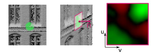
Figure 6.4: Local shape descriptor: For a point we extract all neighbors within a given radius form the point cloud. Given the surface normal n, a tangent frame is computed. Finally, a smooth depth image is generated by splatting all extracted points onto the tangent plane. The right picture shows the noise-reduced result after PCA compression.
