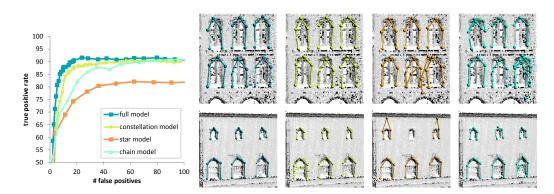
**Figure 7.12:** Evaluation of different model structures. The excerpts show typical results for the different model types. Results are shown for similar numbers of false positives. The colors represent the different models.
