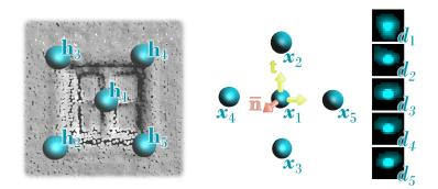
**Figure 7.3:** Each shape *H* is associated with a spatial layout *X* and local shapes  $\mathbf{d}_i$ . The layout is given by relative coordinates  $\mathbf{x}_i$  of the individual parts  $\mathbf{h}_i$  in a coordinate frame centered at the first part. The local shape is a collection of the local shape descriptors of the shape parts.
