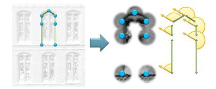
**Figure 6.2:** Example for a window model: The object parts are aligned along the outline of a window. Starting from the lower left corner, we chose distinct parts at edges and corner points. Blue marks the variables in the point cloud space and green the edges of the graphical model. The evidence function  $\phi$  yields matching scores for local shapes and  $\psi$  defines the compability of the parts, i.e. the relative alignment, given a global orientation (yellow arrows).
