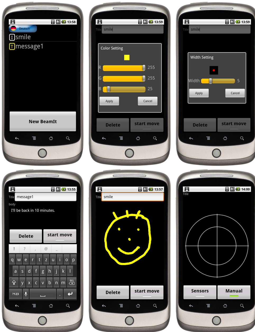
Figure A.4: Screenshots of Beam-It application on Nexus One smartphone: initial window showing a list of previously created Beam-Its, menu for color selection and menu for stroke width adjustment [top row, from left to right]; typed Beam-It content, hand-drawn Beam-It content and the cross pad for position adjustment of the Ubiquitous Cursor [bottom row, from left to right]
