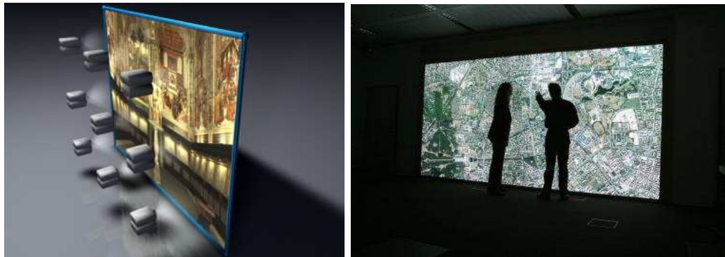
Figure 4.6: HEyeWall: tiled rear-projection setup [left] and resulting projected screen [right] (source: http://www.christianknoepfle.de/projekt_heyewall.htm )
