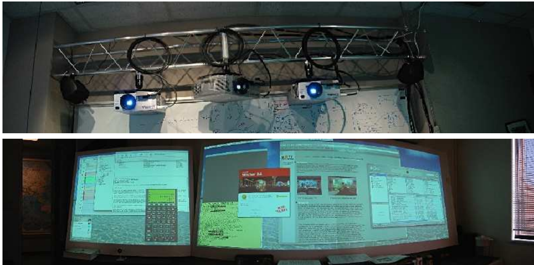
Figure 4.3: Office of “Real Soon Now”: panoramic images of the projector setup [top] and the resulting projected screens [bottom] (source: http://www.cs.unc.edu/~welch/oorsn.html )
