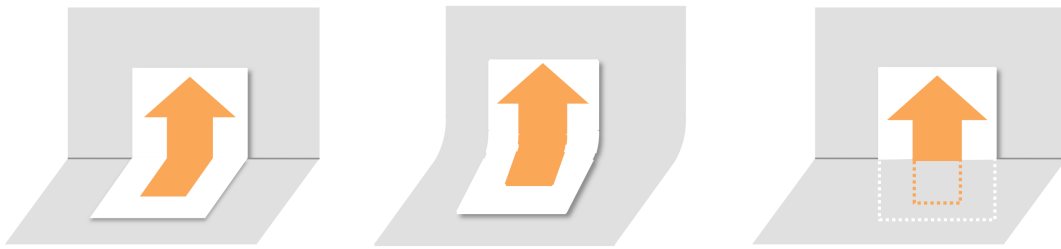
Figure 5.2: Illustration of different discontinuity handling approaches: image bent around a corner [left], image bent along a curve [center] and Virtual Display switching orientation at a corner [right]
