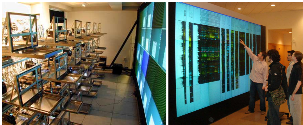
Figure 4.4: Scalable Display Wall: projector setup [left] and resulting projected screen [right] (source: http://www.cs.princeton.edu/omnimedia/ )
