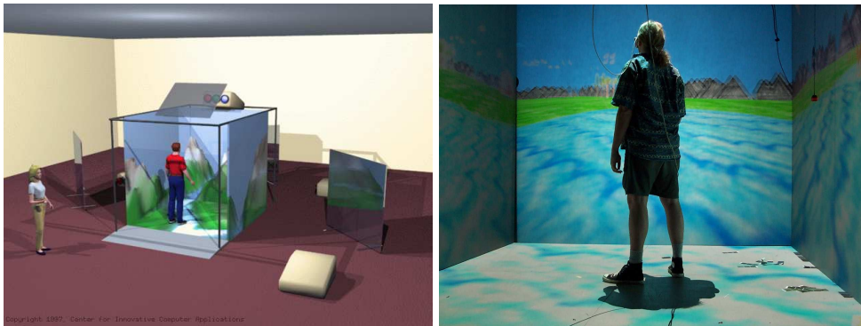
Figure 4.1: A model of a prototypical CAVE setup [left] and a user interacting in the CAVE at EVL [right] (sources: http://www.indiana.edu/~rcapub/v21n2/p28.html and http://de.wikipedia.org/wiki/Cave_Automatic_Virtual_Environment )
