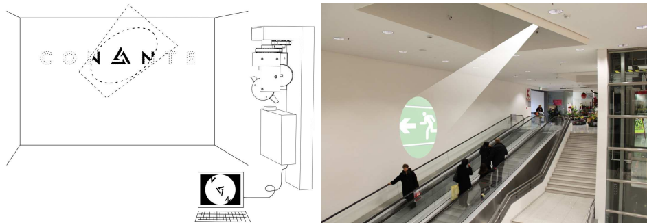
Figure 4.13: LumEnActive: schematic illustration of the system [left] and an exemplary scenario [right] (source: [Rapp and Weber, 2010])
