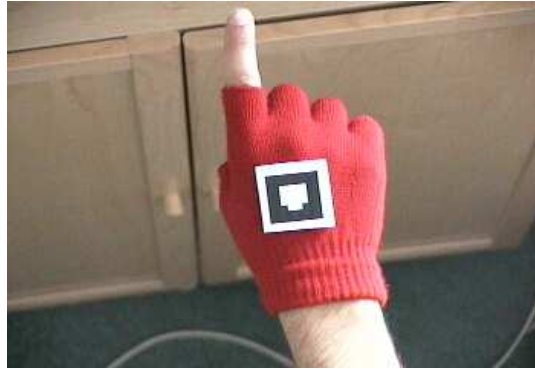
Figure 6.20: Colored glove with ARToolKit marker for recognizing pointing gestures
