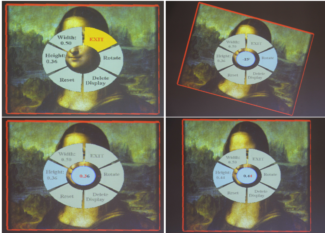
Figure 6.26: Display menu with submenus: main menu [upper left], rotation submenu [upper right], submenu for height adjustment [lower left] and image with modified height [lower right]
