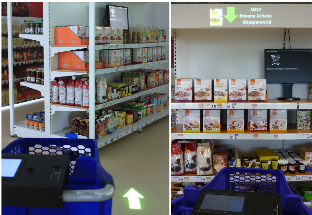
Figure 6.31: Micro navigation hint projected on the floor in front of the SmartCart [left] and in combination with customer-adapted advertising on top of a product shelf [right]
