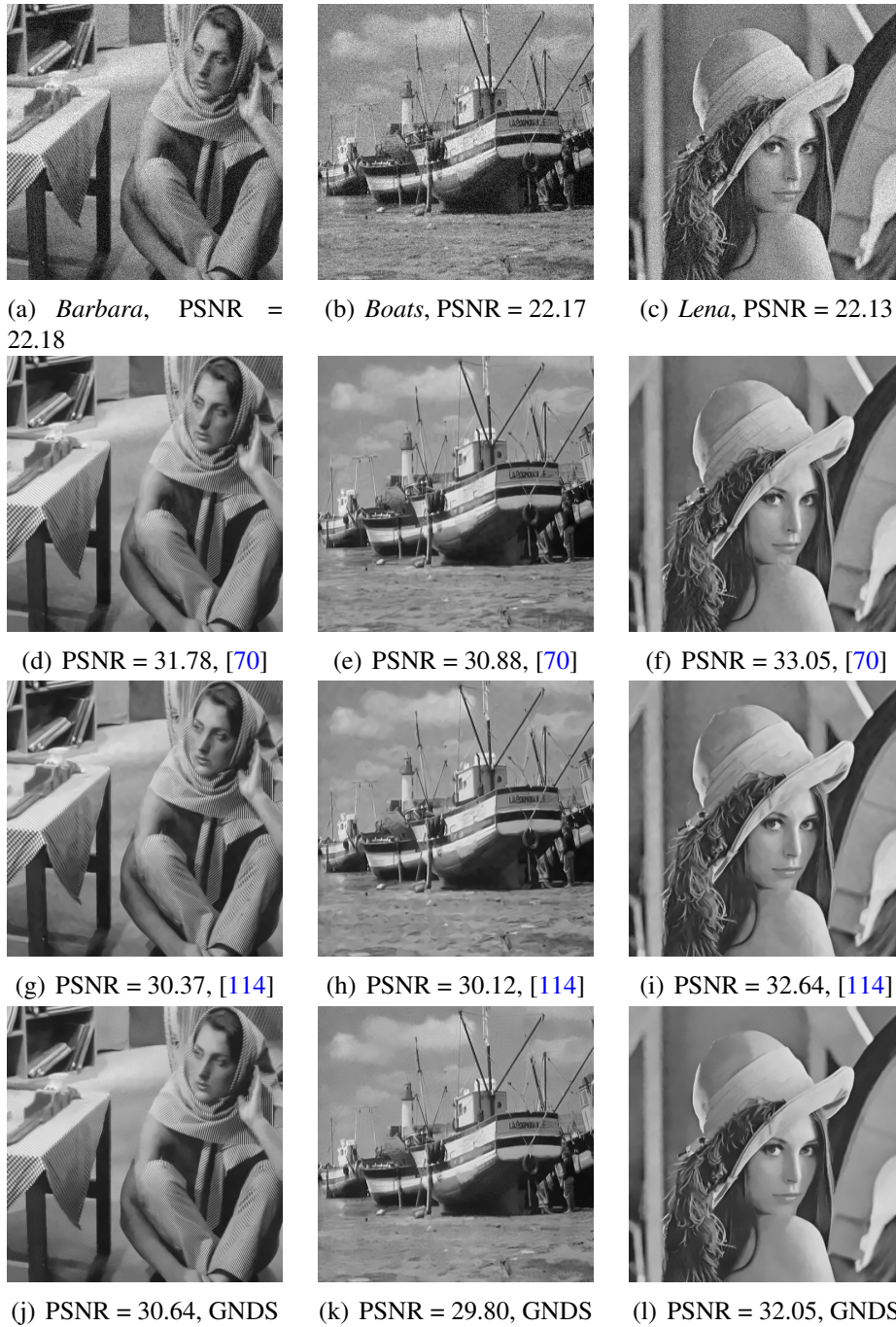
Figure 3.5: Comparison to state-of-the-art methods. Top Row : Test images degraded by Gaussian noise with standard deviation 20. 2nd Row : Restored images by Dabov et al. [70]. 3rd Row : Restored images by Kervrann et al. [114]. Bottom Row : Restored images by the proposed GNDS model (3.2).
