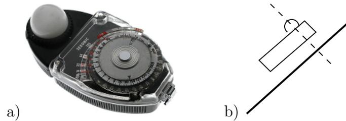
Figure 7.3: A Photographers Incident Lightmeter. **a)** The white diffuser hemisphere is used to integrate the incident light. A single sensor element under the hemisphere converts the light level to an electric voltage. The scale gives a readout in photometric units. A dial allows calibration for film speed. **b)** To take a measure of the light illuminating a plane, the lightmeter is held parallel to the plane.
