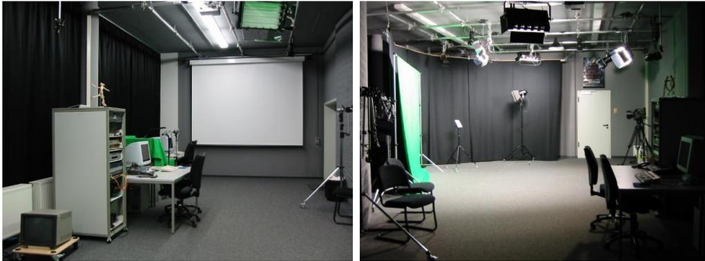
*Figure E.1: The (Mixed Reality) Studio Lab at the Computer Graphics Department at Saarland University. A high ceiling headroom, a mounting grid for lighting fixtures, cameras and chroma green backdrops simplify mixed reality experiments.*
