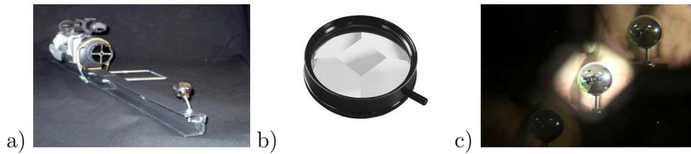
Figure 7.17: **a)** The ICT real-time lightprobe consisting of a consumer video camcorder, a small mirror ball, an optical effect prism and ND filter gels. **b)** An effect prism filter to achieve multiple images. **c)** One frame of the recorded video. A post-process generates a HDR lightprobe video. (Photos a+c Courtesy of ICT, Jamie Waese)
