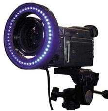
*Figure 5.2: The Lighting device for the BBC Truematte technology. A ring of colored LEDs on the camera lens in combination with a highly retro-reflective backdrop fabric provides a nearly perfect chroma keying method.*
