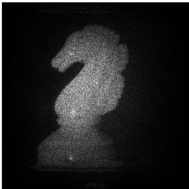
**Figure 2.4:** Numerical reconstruction of a digital phase shift hologram depicting a chess knight. Distance between model and hologram plane was  $0.46\text{ m}$  and the hologram has a size of  $512 \times 512$  pixels. Each pixel has a size of  $9\ \mu\text{m}$ . Note the speckle pattern as the irregular structure over the hologram.
