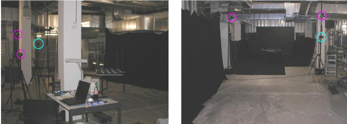
Figure 6.24: **Ball acquisition setup.** Left: a stereo camera pair (encircled in magenta) facing the black curtain on the right is capturing the ball’s initial flight parameters. The ball is illuminated by a stroboscope (cyan). Right: a stereo camera pair (magenta) and a strobe light (cyan) facing towards the black carpet in the back are responsible for capturing the ball trajectory close to the “home base”. See Figure 6.22 (bottom) for a schematic illustration of the setup.
