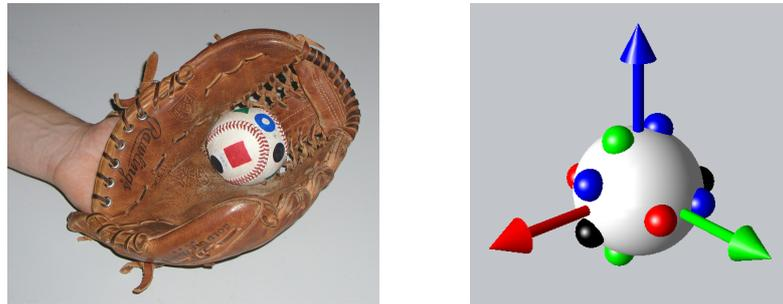
Figure 6.28: **Ball with markers.** Left: baseball equipped with optical markers in pitcher's glove. Right: illustration of the ball's coordinate system. Markers are depicted as small colored spheres on the ball.
