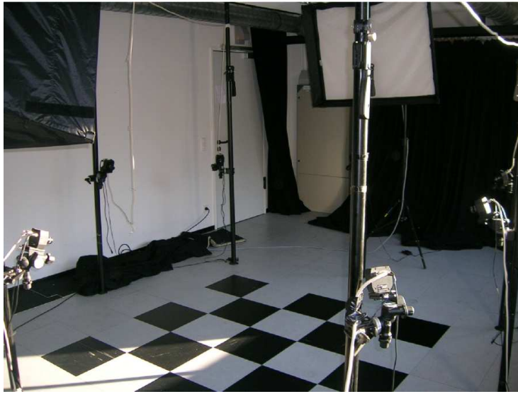
Figure 4.9: Camera setup using eight cameras and two HMI lamps with softboxes.
