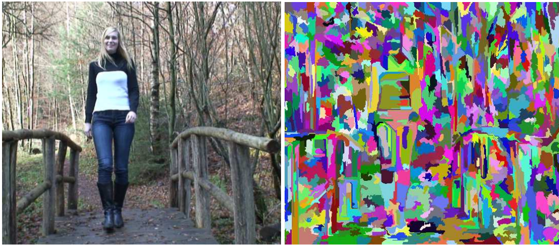
Figure 6.3: Result of segmentation during preprocessing. Left: input image, right: segmentation result, each colored region is a superpixel.
