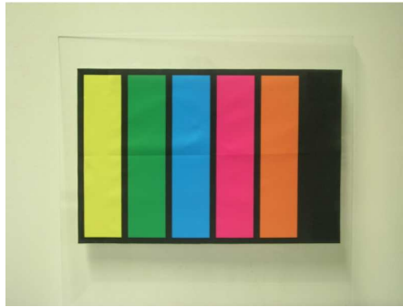
Figure 4.4: Test pattern with five colors for color hue calibration.
