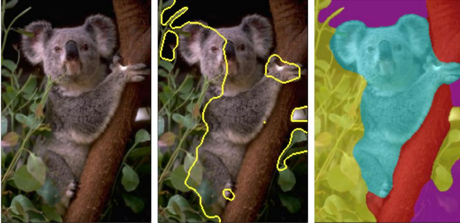
**Fig. 5.58:** LEFT: Input image ( $169 \times 250$ ). CENTER: Two-region segmentation. RIGHT: Multi-region segmentation, 4 regions have been detected.
