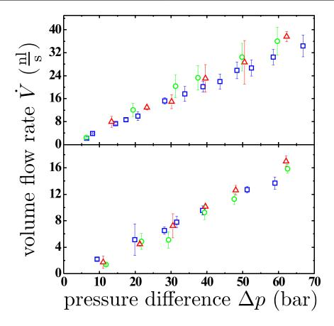
**Figure 10.3.:** Volume flow rates  $\dot{V}$  of n-hexane in V10 (upper panel) and V5 (lower panel) as a function of the applied external pressure difference  $\Delta p$  at three different temperatures: 25 °C ( $\square$ ), 40 °C ( $\bigcirc$ ), and 50 °C ( $\triangle$ ).
