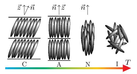
**Figure 8.8.:** Illustration of common liquid crystal phases. Upon heating a frozen liquid crystal one might pass the following mesophases: smectic C (C), smectic A (A), and nematic (N). Beyond the clearing point  $T_c$  the liquid crystal is in the isotropic state (I).
