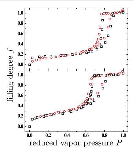
**Figure B.3.:** Nitrogen sorption isotherms at T = -196 °C on untreated ( $\square$ ) and silanized ( $\bigcirc$ ) V10 (upper panel) and V5 (lower panel), respectively.
