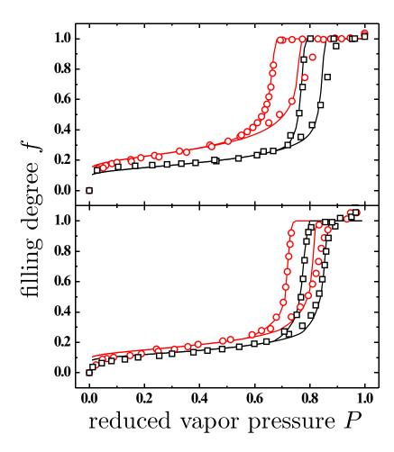
Figure B.2.: Nitrogen (upper panel) and water (lower panel) sorption isotherms on V10 ( $\square$ ) and V5 ( $\bigcirc$ ) carried out at T = -196 °C and T = 4 °C, respectively. Solid lines are fits according to a mean field model (Saam-Cole).
