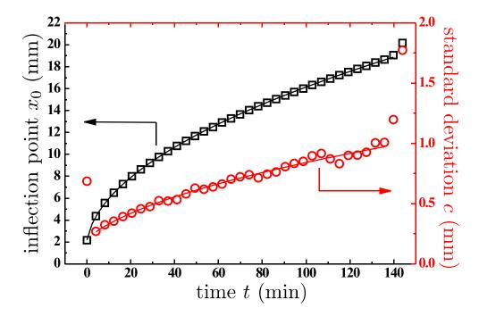
Figure 6.4.: Inflection point  $x_0$  ( $\square$ ) and standard deviation c ( $\bigcirc$ ) from fits of Eq. (6.4) to the profiles partly shown in Fig. 6.3 as a function of the time t. The inflection point may be identified as the mean front position of water invading the sealed V10 sample whereas c quantifies its washout. Please note that different scalings are used. The lines are  $\sqrt{t}$ -fits to the underlying data. The data density is reduced by a factor of 5.
