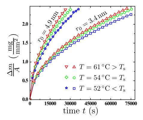
**Figure 8.4.:** Specific mass uptake of both V5 and V10 due to n-tetracosane imbibition as a function of the time for selected temperatures close to, but above the bulk freezing temperature. Solid lines correspond to  $\sqrt{t}$ -fits. The data density is reduced by a factor of 1000.
