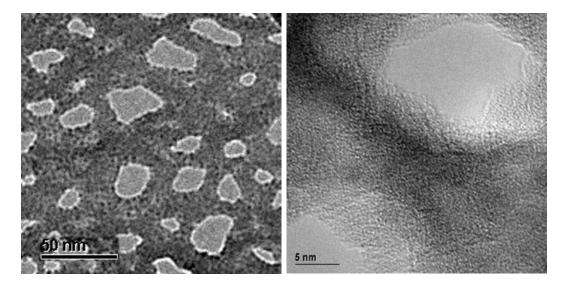
**Figure 3.6.:** Transmission electron micrographs of porous silicon with different magnification factors. The sample was thinned by means of Ar ion milling in order to ensure a sufficient electron transmission rate. The pores correspond to the bright areas. Courtesy of Jörg Schmauch, Saarland University, Saarbrücken, Germany.
