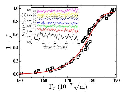
Figure 7.7.: Inverse filling degree 1-f as a function of the imbibition strength  $\Gamma_{\rm r}$  ( $\square$ ) for n-tetradecane invading V10. The solid line is a polynomial fit to the underlying data set, which is used for an analytical investigation of the  $f(\Gamma_{\rm r})$ -relation. Inset: Selected rise level curves  $h_f(t)$  for given filling degrees f normalized by  $h_{f=0.5}(t)$ . The respective filling degrees are listed within the plot.
