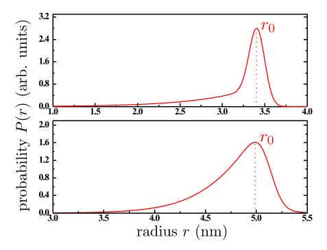
**Figure 3.2.:** Distribution of pore radii as extracted from nitrogen sorption isotherm measurements for both V5 (upper panel) and V10 (lower panel). The peak values of the mean pore radii  $r_0$  (3.4 nm and 4.9 nm) are indicated by the dotted lines. For more details see Appendix B.
