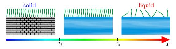
**Figure 8.1.:** Illustration of the surface freezing transition. Between the bulk melting point  $T_{\rm f}$  and the phase transition temperature  $T_{\rm s}$  one single solid monolayer is established on the free surface of the liquid.
