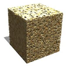
**Figure 3.1.:** Raytracing illustration of the sponge-like internal structure of a porous Vycor<sup>®</sup> cuboid with its tortuous pore network.
