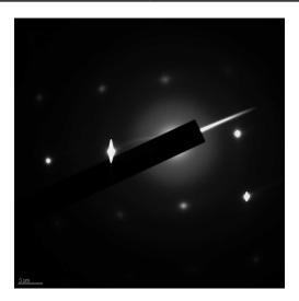
**Figure B.4.:** Diffraction pattern of porous silicon taken in the TEM setup. Courtesy of Jörg Schmauch, Saarland University, Saarbrücken, Germany.
