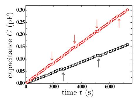
**Figure 10.4.:** Illustration of frequent drops (see arrows) in the raw data signal C(t) of the forced imbibition measurements of n-hexane in V10 at 25 °C due to the raise of bubbles of translocating gas. The applied pressure differences are 35 bar ( $\square$ ) and 68 bar ( $\bigcirc$ ). The data density is reduced by a factor of 10.
