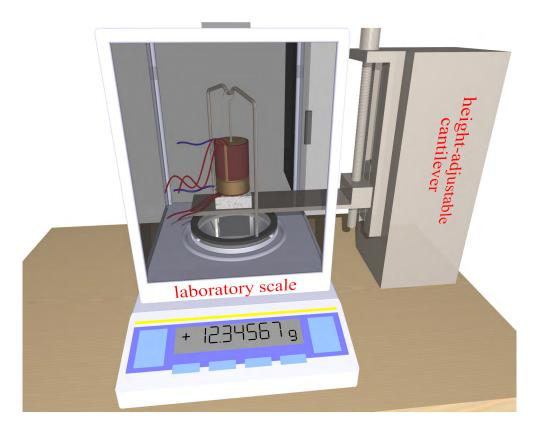
Figure 5.1.: Raytracing illustration of the liquid imbibition setup (LIS). The cell (see Fig. 5.2) is mounted on a height-adjustable cantilever reaching into the housing of a standard laboratory scale from Sartorius (model: BP211D).
