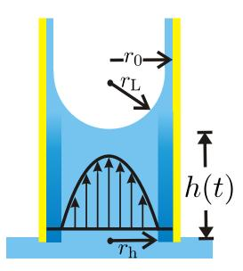
**Figure 4.4.:** Schematic view of the capillary rise in a cylindrical pore with pore radius  $r_0$ , Laplace radius  $r_L$  and hydrodynamic pore radius  $r_h$ .
