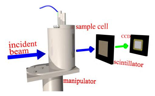
**Figure 5.4.:** Raytracing illustration of the structural principle of the neutron radiography setup ANTARES located at the research reactor FRM II of Technische Universität München in Garching, Germany. For a detailed view into the sample cell see Fig. 5.5. Blue arrows indicate neutron radiation, the green arrow indicates visible light.
