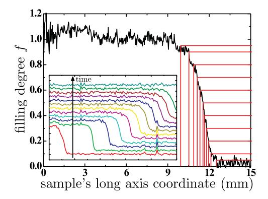
**Figure 7.6.:** Illustration of the evaluation method of the normalized gray scale value profiles obtained from neutron radiography measurements of n-tetradecane invading V10. The shown grid corresponds to the following filling degrees f: 5%, 10%, 20%, ..., 80%, 90%, 95%. Inset: Series of normalized gray scale value profiles of n-tetradecane invading porous Vycor<sup>®</sup> (identically equal to Fig. 6.3).
