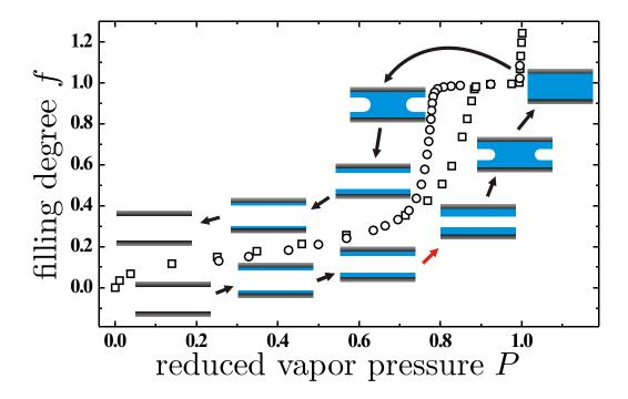
**Figure B.1.:** Nitrogen adsorption ( $\square$ ) and desorption ( $\bigcirc$ ) isotherm on porous silicon at  $T = 77\,\mathrm{K} = -196\,^{\circ}\mathrm{C}$ . The insets illustrate the corresponding behavior of the condensate in a cylindrical pore. The red arrow indicates the non-equilibrium step of the buildup of metastable layers at the pore walls.
