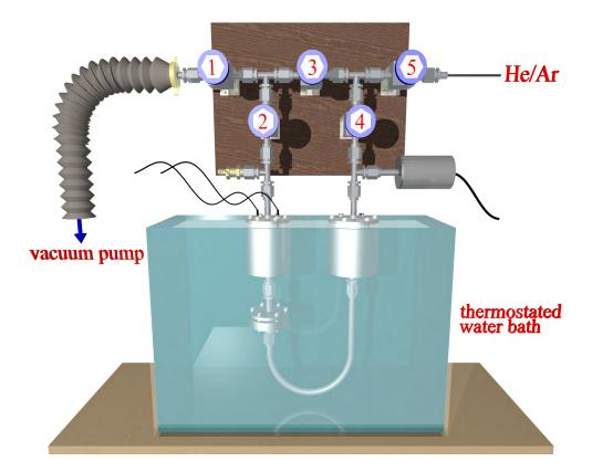
**Figure 9.1.:** Raytracing illustration of the membrane flow apparatus (MFA) consisting of a gas handling and the actual flow system. The latter is temperature-controlled in a water bath (for a more detailed view see Fig. 9.2). The gas handling can be evacuated by a vacuum pump and can be filled with helium or argon gas. The setup was partly constructed in the course of the diploma thesis of Stefanie Greulich [141].
