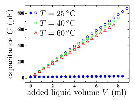
**Figure 9.3.:** Calibration measurements of the cylindrical capacitor for water (open symbols) and n-hexane (filled symbols) at selected temperatures. The capacitance C was measured as a function of the liquid amount V filled into the capacitor. For the empty capacitor it is  $C \approx 15 \,\mathrm{pF}$ .
