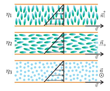
**Figure 8.9.:** The experimental Couette flow conditions for measurements of the three Miesowicz shear viscosity coefficients of nematic liquid crystals:  $\eta_1$  for  $\vec{n} \perp \vec{v}$  and  $\vec{n} \parallel \nabla v$ ,  $\eta_2$  for  $\vec{n} \parallel \vec{v}$  and  $\vec{n} \perp \nabla v$ ,  $\eta_3$  for  $\vec{n} \perp \vec{v}$  and  $\vec{n} \perp \nabla v$ .
