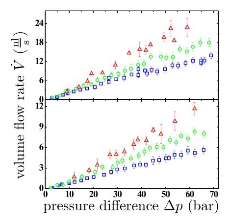
**Figure 10.2.:** Volume flow rates V of water in V10 (upper panel) and V5 (lower panel) as a function of the applied external pressure difference  $\Delta p$  at three different temperatures:  $25 \,^{\circ}\text{C}$  ( $\square$ ),  $40 \,^{\circ}\text{C}$  ( $\bigcirc$ ), and  $60 \,^{\circ}\text{C}$  ( $\triangle$ ).
