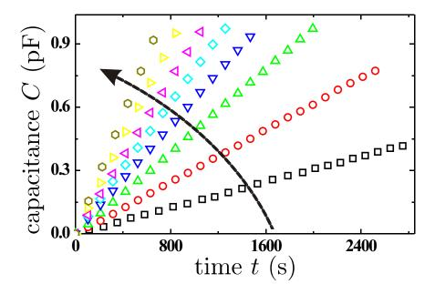
Figure 10.1.: Time dependent variation in the capacitance C of the cylinder capacitor due to the flow of water through V10 at 25 °C for a series of applied external pressures. The arrow indicates the direction of increasing  $\Delta p$ . The shown measurements correspond to: 8 bar, 16 bar, 24 bar, 31 bar, 37 bar, 45 bar, 54 bar, and 70 bar. The data density is reduced by a factor of 20.
