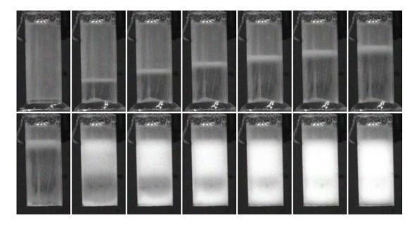
Figure 4.5.: Series of pictures of a detachment experiment of water invading a porous Vycor® block (V10,  $V_s = 6.75 \times 4.85 \times 16.70 \,\mathrm{mm^3}$ ) at room temperature. Top and side facets were sealed. (first row): Standard imbibition with white advancing front. Duration between each picture:  $10 \,\mathrm{min}$ . (second row): Detachment from the reservoir and turning white of the filled parts. Intervals between pictures:  $30 \,\mathrm{min}$ .
