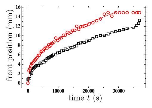
Figure 7.4.: Time dependent upper  $(\bigcirc)$  and lower  $(\Box)$  bound position of the front extracted from the profiles partly shown in Fig. 7.3. The lines are  $\sqrt{t}$ -fits to the underlying data. The data density is reduced by a factor of 20.
