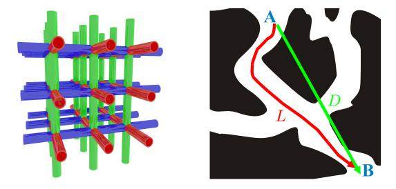
**Figure 2.1.:** Illustration of the meaning of the tortuosity  $\tau$  of a pore network such as Vycor<sup>®</sup>. (left): For an isotropic distribution of the pores only every third pore is subjected to the pressure gradient yielding  $\tau = 3$ . (right): For meandering pores an additional factor of  $\frac{L}{D}$  must be introduced to correct the length D of the direct interconnection of two points for the actual path length L.
