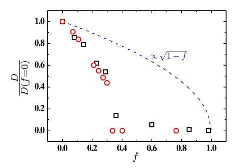
**Figure B.7.:** Diffusion coefficients D at  $T=40\,\mathrm{K}$  of helium flowing through V5  $(\Box)$  and porous silicon  $(\bigcirc)$  as a function of the filling degree f of argon. The coefficients are normalized with respect to D(f=0). The measurements on V5 were carried out by Stefan Bommer in the course of his diploma thesis (see [2]).
