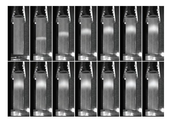
**Figure 5.3.:** Series of pictures of a pinning experiment of water invading a porous Vycor<sup>®</sup> block (V10,  $V_s = 8.14 \times 6.05 \times 29.00 \,\mathrm{mm}^3$ ) at room temperature. The sample is not sealed. Intervals between pictures: 106 min. Due to the increasing impact of evaporation the front is eventually pinned.
