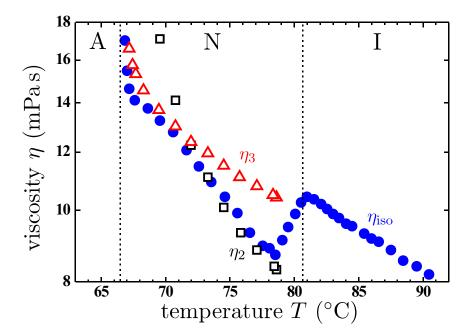
Figure 8.10.: Miesowicz shear viscosities  $\eta_2$  ( $\square$ ) and  $\eta_3$  ( $\triangle$ ) of the liquid crystal 8OCB compared to its free flow viscosity  $\eta_{\rm iso}$  ( $\bullet$ ) according to [125].
