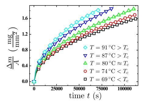
Figure 8.11.: Specific mass uptake of V5 due to the imbibition of the liquid crystal 8OCB as a function of the time for selected temperatures below and above the clearing point  $T_c \approx 80$  °C. Solid lines correspond to  $\sqrt{t}$ -fits. The data density is reduced by a factor of 2500.
