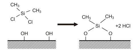
**Figure 3.3.:** Illustration of the reduction of the surface energy through silanization. In the presence of dimethyldichlorosilane  $(Si(CH_3)_2Cl_2)$  the polar and consequently high-energy hydroxyl (OH) groups at the glass surface are replaced by low-energy methyl (CH<sub>3</sub>) groups.
