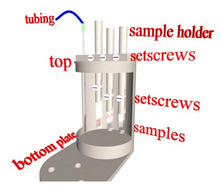
**Figure 5.5.:** Raytracing illustration of a view into the sample cell of the neutron radiography setup depicted in Fig. 5.4. The whole cell and the sample holder are made of aluminum. The samples are mounted on the clamp-like sample holder. Up to three of them can simultaneously be attached to the cell. The liquid is supplied via a tubing employing an external pump.
