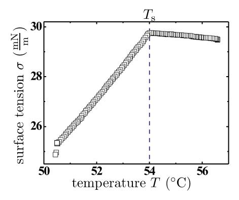
**Figure 8.3.:** Surface tension  $\sigma$  of bulk n-tetracosane as a function of the temperature T as deduced from Wilhelmy plate measurements. Courtesy of Moshe Deutsch, Bar-Ilan University, Ramat-Gan, Israel.
