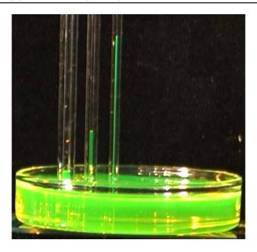
**Figure 4.2.:** Final state of the capillary rise process of dyed water in three glass capillaries with different diameters. Applying Jurin's law Eq. (4.4) one can deduce the capillary's diameter  $r_0$  from the maximum rise level  $h_{\text{max}}$ . Courtesy of Hans Peter Läser, Soil Physics, Institute of Terrestrial Ecology, ETH Zürich, Swiss.
