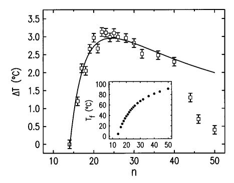
Figure 8.2.: The temperature range of existence  $\Delta T = T_{\rm s} - T_{\rm f}$  for the surface crystalline phase as a function of the chain length in terms of the number of carbon atoms n in the hydrocarbon backbone. The solid line is a theoretical expression derived in Ref. [109], and the inset charts the bulk freezing temperatures  $T_{\rm f}$  vs n. Courtesy of Moshe Deutsch, Bar-Ilan University, Ramat-Gan, Israel.
