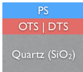
Figure 6.1: Schematic of the prepared dewetting system: A polystyrene film floated on a silanized quartz wafer.
