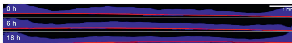
Fig. 4. Raman cross section images of the entire membrane diameter depicting lipid coating (blue) on the supportive membrane (red) prior to (0 h), after 6 h and 18 h of investigating coating resistance against media under dynamic flow conditions. Due to image size the free aspect ratio was deregulated for better visualization. (For interpretation of the references to color in this figure legend, the reader is referred to the web version of this article.)
