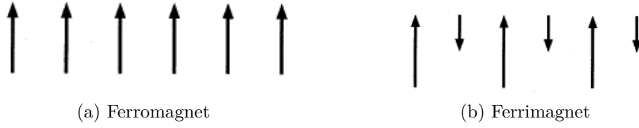
Figure 2.1.: Exchange coupling for ferromagnets and ferrimagnets. Image modified from [18]
