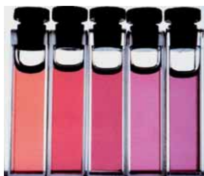
Figure 2.5: Color change due to a different medium - Changing in the plasmon peak position induced by varying the solvent refractive index. Refractive indices of the solutions at the absorption band maximum are 1.336, 1.407, 1.481, 1.525 and 1.583, respectively. Image from Underwood and Mulvaney [41]
