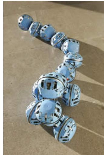
(b) An ATRON re-configurable modular robotic organism
