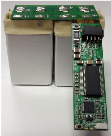
(a) Battery pack electronics front side
