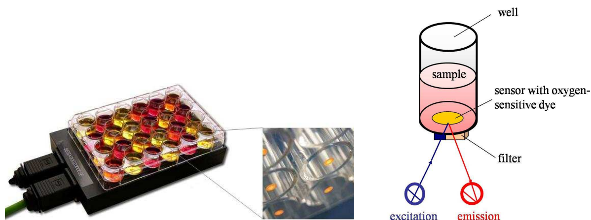
A Figure 3.2: Assembling of the SensorDish ® Reader (SDR). (A) SDR with an OxoDish ® plate on top. Sensor spots are immobilised at the bottom of each well. (B) Measurement principle of the SDR. The sensor is excited by the reader non-invasively through the transparent bottom of the OxoDish ® plates. Its emission is detected from the bottom side as well. Images were received from PreSens (Regensburg, Germany).
