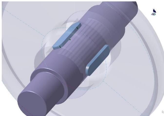
Figure 6: 3D-CAD-model of the shaft to collar connection
