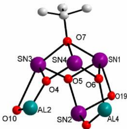
Figure 24: Representation of the coordination environment around the tin atoms.
