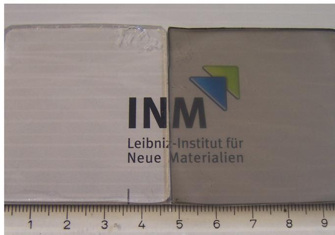
**Fig. 6.41:** Photograph comparing the transparency of  $TiO_2$  (left) and  $TiO_2$ /MWNT nanocomposites containing 3 mg/ml MWNTs (right).
