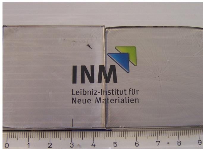
**Fig. 6.17:** Photograph comparing the optical transparency of MWNT-NET (left) and MWNT-NET-Si (right) deposited on borosilicate glass at 350 °C.
