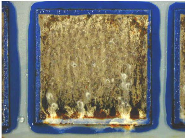
Figure 3.180: Sputtered zinc titanium coating ZTi<sub>98</sub> (+9.4 at.% Ti) after 480 h SST
