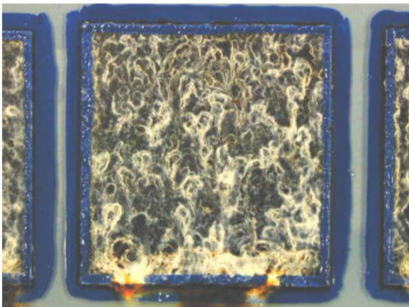
Figure 3.176: Sputtered zinc chromium coating ZCr 3<sub>8</sub> (+3.1 at.% Cr) after 480 h SST
