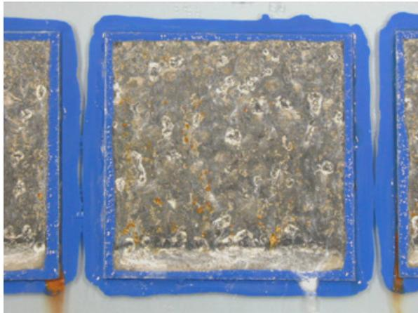
Figure 3.178: Sputtered zinc titanium coating ZTi<sub>18</sub> (+1.7 at.% Ti) after 119 h SST
