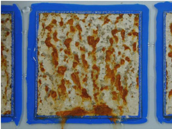
Figure 3.168: Thin sputtered  $ZB_8$  zinc coating after 9 h SST
