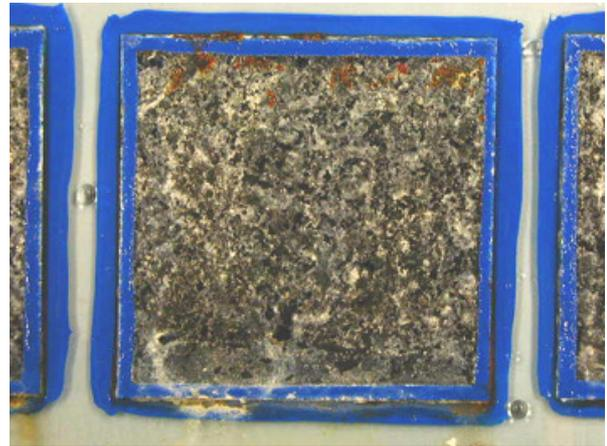
Figure 3.169: Sputtered zinc aluminium coating  $ZA12_8$  (+2.6 at.% Al) after 446.5 h SST
