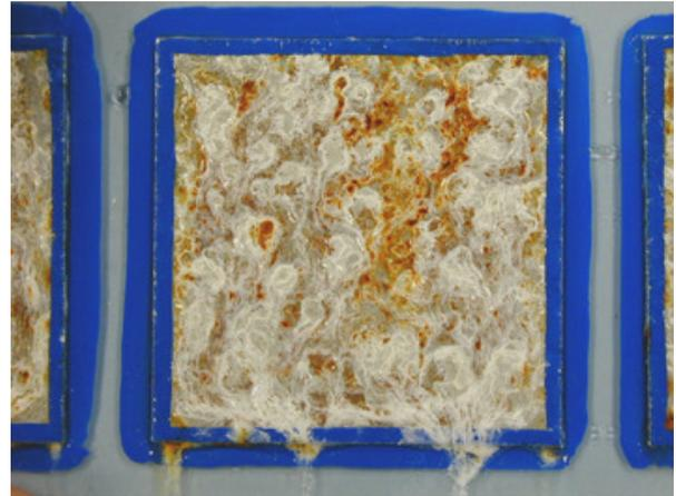
Figure 3.167: Sputtered zinc coating  $ZC_8$  after 62 h SST
