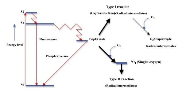
Figure 4. Jablonski diagram representing the excitation and relaxation of a photosensitizer (PS), with type I and type II photoreactions.
