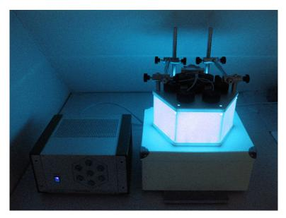
**Figure 5.** Illumination box ( $\lambda = 370$  nm, 2 J/cm<sup>2</sup>)
