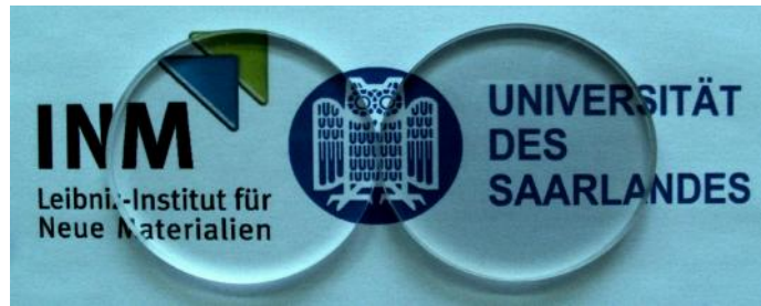
Figure 5.27: Optical image of non-coated (left) and coated (right) glass plates.
