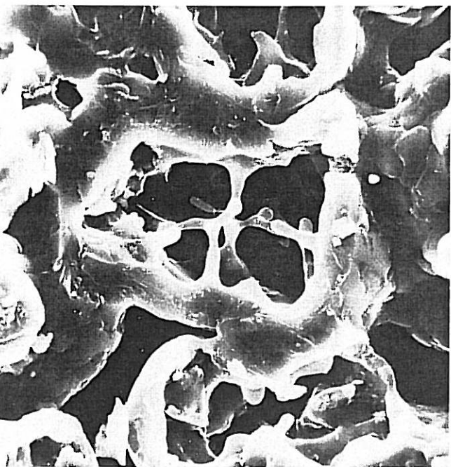
Fig. 4. High-porosity beryllium alloy produced from cobalt-coated beryllium particles by sintering 1000\times . (From ALDINGER [1974].)
